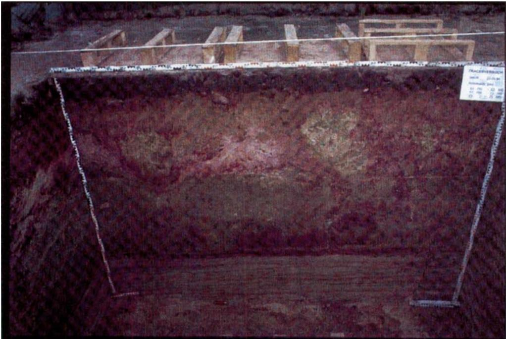
**Fig. 1.2:** Preferential flow paths in a highly variable soil of a push moraine. The flow region is colored by Rhodamine applied during a tracer experiment.
