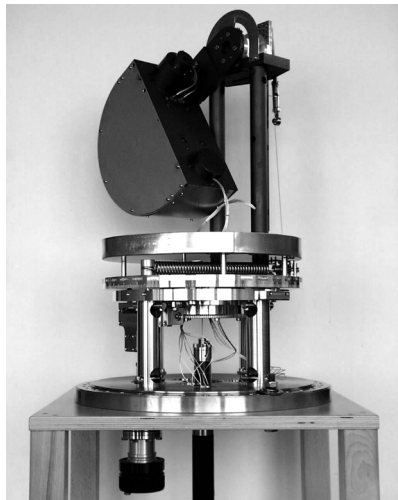
Figure 5.3: The ASPHERE spectrometer of the University of Kiel. The hemispherical analyzer is mounted on a two-axis goniometer.
