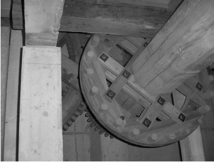
Figure 4: Gear Transmission of Le Tsáblo. Left: Gear on the First Shaft, which carries the Waterwheel. Right: Second Horizontal Shaft with One of the Two Wheels with Lateral Teeth.
