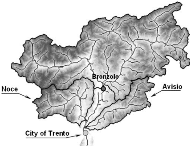
Figure 1: Description of the Adige River Basin up to Trento and its Major Tributaries: Avisio, Noce, and Bronzolo's Watersheds. (Map Obtained Using a Digital Elevation Model of 240-M Resolution.)
