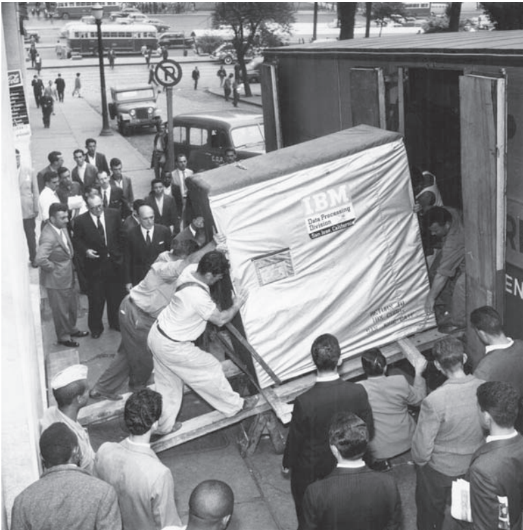
Fig. 2.2 The world's first disk drive. The RAMAC 305, developed by IBM in 1956, had a storage capacity of 5 MB. (From IBM Corporate Archives)
