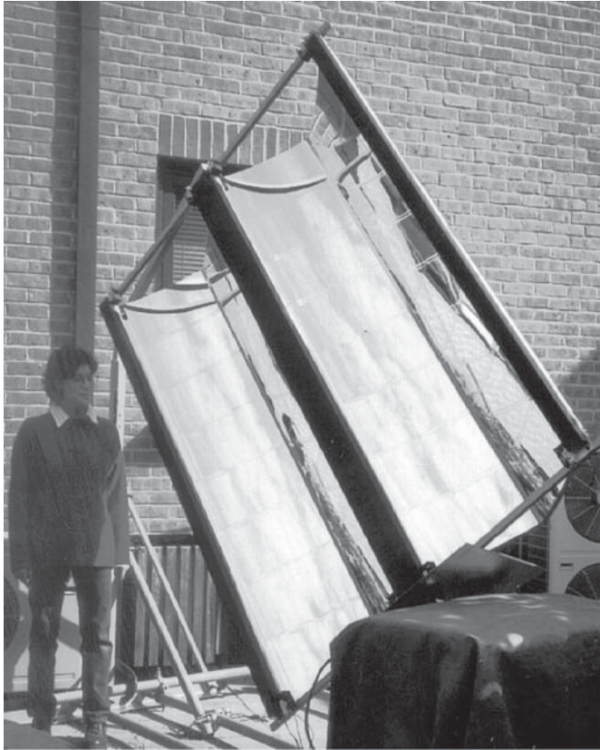
Figure 13.42 SMTS concentrator for C_g = 30\times and an acceptance angle \pm 1.5^\circ .
