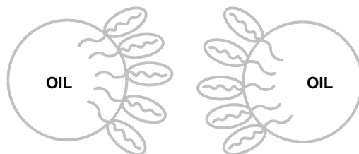
Fig. 7.6 The hydrated polyoxyethylene chains provide a steric barrier between approaching oil droplets in o/w emulsions.
