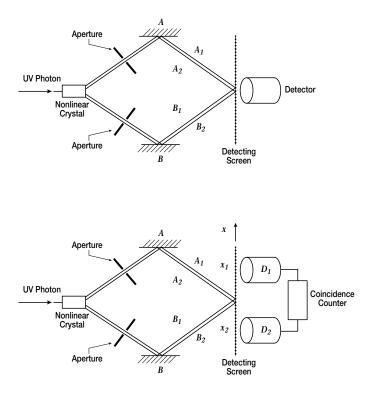
In the experiment above, a nonlinear crystal is pumped by a laser, producing pairs of entangled photons. Since the photon that enters the crystal can produce a pair of photons in any of infinitely many ways (because all that's required is that the sum of the frequencies of the progeny be equal to the frequency of the parent photon), within a certain range of distance on the screen there can be found photons that are entangled with each other.
