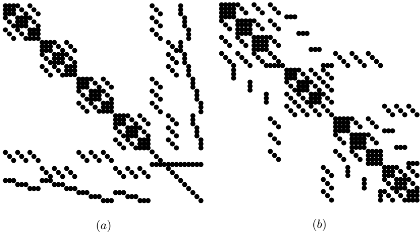
Figure 4.6.7. Two topological structures of L_C , the orthogonal collocation matrix on a 2 \times 2 multidomain, depending on the ordering of the unknowns (see text). In this example, the polynomial expansion in each subdomain has N = 5 .
