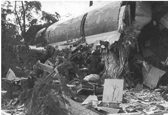
Figure 4.1 The aftermath of Flight 173. It is generally agreed that poor crew resource management was contributory to the crash. The lack of fire damage is due to the absence of fuel at the time of the crash.
