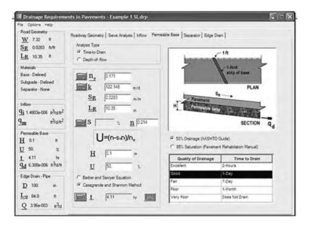
Figure 4.5 Checking the base design by the time-to-drain method.
