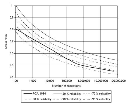
Figure 6.1 Comparison of PCA 1984 and StreetPave fatigue relationships.
