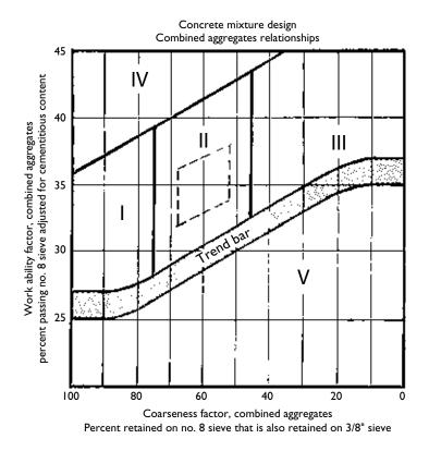
Figure 5.1 Combined aggregate relationship (coarseness factor) chart (courtesy: Shilstone and Shilstone 2002).
