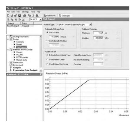
Figure 15.4 Properties of rough asphalt concrete subbase.
