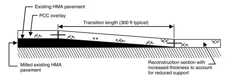
Figure 18.6 A transition detail for bridge approaches and overpasses for whitetopping (figure courtesy: ACPA, Smith et al. 2002: 5–9).
