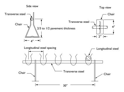
Figure 12.1 Combination chair and transverse steel detail (1 in = 25.4 mm) (FHWA 1990b).
