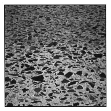
Figure 3.8 Polished aggregate surface (Miller and Bellinger 2003: 49).
