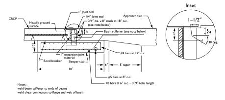
Figure 12.3 Recommended WF steel beam terminal joint design (1 in = 25.4 mm, 1 ft = 305 mm) (FHWA 1990b).
