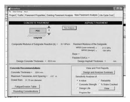
Figure 9.5 Concrete pavement design.
