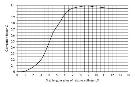
Figure 7.1 Curling stress correction factors for a finite slab (after Bradbury 1938).
