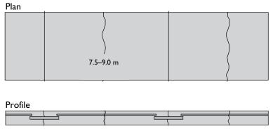
Figure 2.2 Jointed reinforced concrete pavement (JRCP) (courtesy: ACPA).
