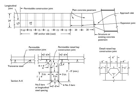
Figure 12.2 Lug anchor treatment (1 in = 25.4 mm, 1 ft = 305 mm) (FHWA 1990b).
