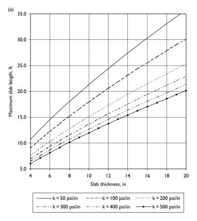
Figure 7.3 Maximum joint spacing based on slab thickness D and modulus of subgrade reaction k for  $L/\ell \le 5.0$  in (a) U.S. customary units and (b) metric units.
