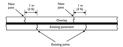
Figure 18.1 Joint mismatching (Smith et al. 2002: 4-9).
