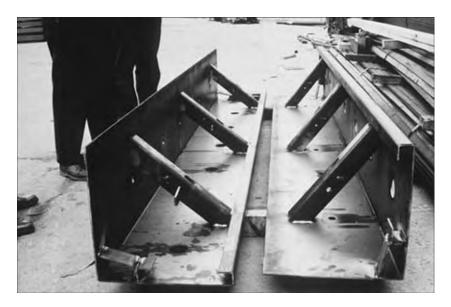
Figure 14.10 Steel forms for fixed form paving (ACPA 1996a: VI-72).
