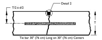
Figure 2.7 Longitudinal joint (FAA 2004).
