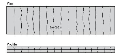
Figure 2.3 Continuously reinforced concrete pavement (CRCP) (courtesy: ACPA).
