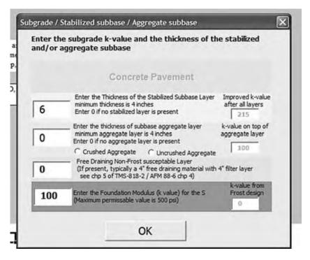
Figure 10.3 FAA R805FAA.xls rigid airport pavement design spreadsheet computation of composite k-value.
