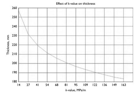
Figure 9.8 Sensitivity of slab thickness to k-value.
