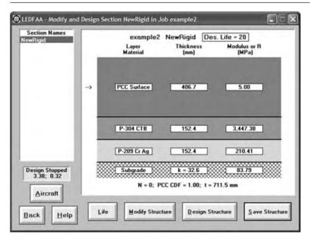
Figure 10.8 Example problem rigid pavement section as designed.
