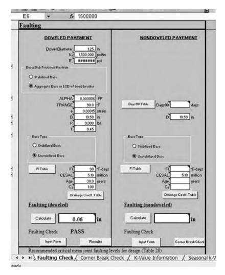
Figure 8.3 Spreadsheet faulting check for AASHTO 1998 design.
