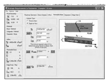
Figure 4.4 Designing the base by the depth-of-flow method.
