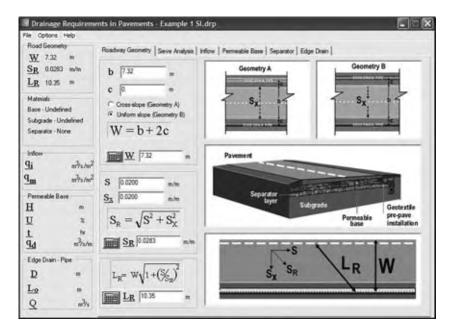
Figure 4.1 Roadway geometry inputs for concrete pavement drainage design.
