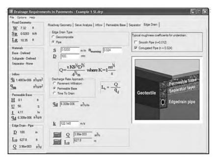
Figure 4.8 Edge-drain design.
