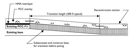
Figure 18.4 A transition detail for bridge approaches and overpasses for unbonded overlays (Smith et al. 2002: 4-13).
