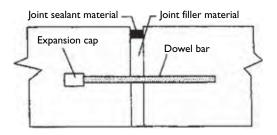
Figure 2.9 Expansion joint detail (FHWA 1990a).
