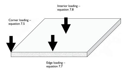
Figure 7.2 Corner, edge, and interior loading.
