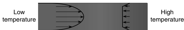
FIGURE 50.17 Schematic representation of the concentration of ionic species in temperature gradient focusing. 49
