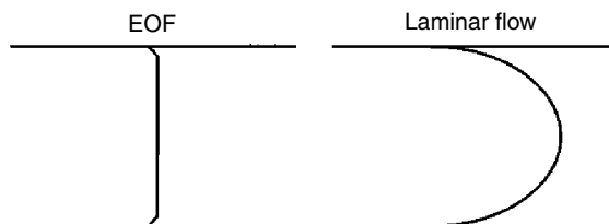
FIGURE 5.2 Flow profiles of EOF and laminar flow.
