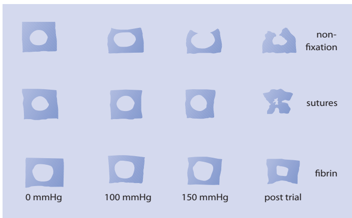
■ Fig. 22.5. Face of contact between mesh (Ultrapro®) and abdominal wall following different fixation techniques (non-fixation vs. eight single sutures vs. fibrin glue). Mesh in a sublay position bridging a 3-cm defect by a 1.5-cm overlap
