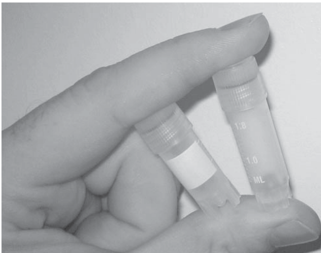
Figure 6.2 Photographs of two plastic ampoules used to freeze and store aliquots of human semen during sperm banking. After filling, the ampoule is sealed with a screw top. Two different sizes of ampoules are shown holding 1.0 ml (left) and 2.0 ml (right) of semen respectively
