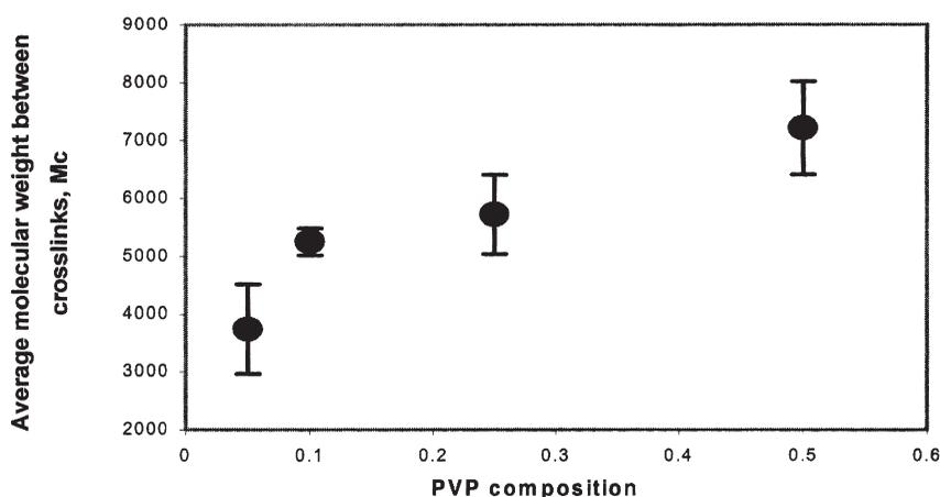
**Fig. 3.** The molecular weight between crosslinks increased for hydrogels with more PVP initially blended into the system, indicating the presence of fewer physical crosslinks.
