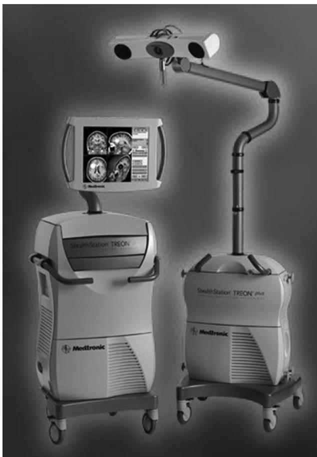
**Fig. 3.** Typical optoelectric navigational system. The Stealth system (courtesy of Medtronic Sofamor Danek, Memphis, TN) is depicted with the optical tracking apparatus and the intraoperative computer imaging display.
