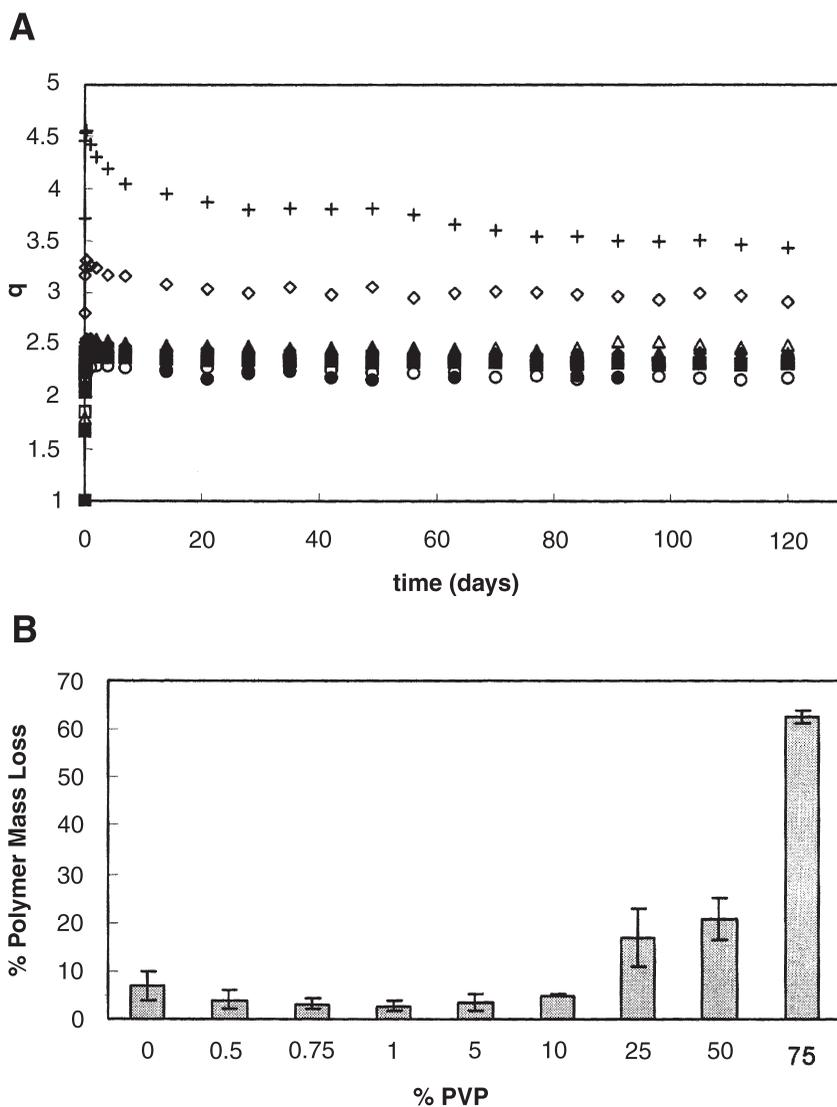
**Fig. 1.** (A) Mass swelling ratio over time of immersion for gels prepared with (A) 143K PVA/10K PVP molecular weight combination with (●) 0% PVP, (○) 0.5% PVP, (■) 0.75% PVP, (□) 1% PVP, (▲) 5% PVP, (△) 10% PVP, (◆) 25% PVP, and (◇) 50% PVP (+) 75% PVP and (B) 50% PVA/50% PVP hydrogel prepared with (●) 143K PVA/10K PVP (○) 143K PVA/40K PVP (■) 95K PVA/10K PVP, and (□) 95K PVA/40K PVP. (B) Polymer mass loss is minimized from that of PVA alone with the addition of 0.5–5% PVP.
