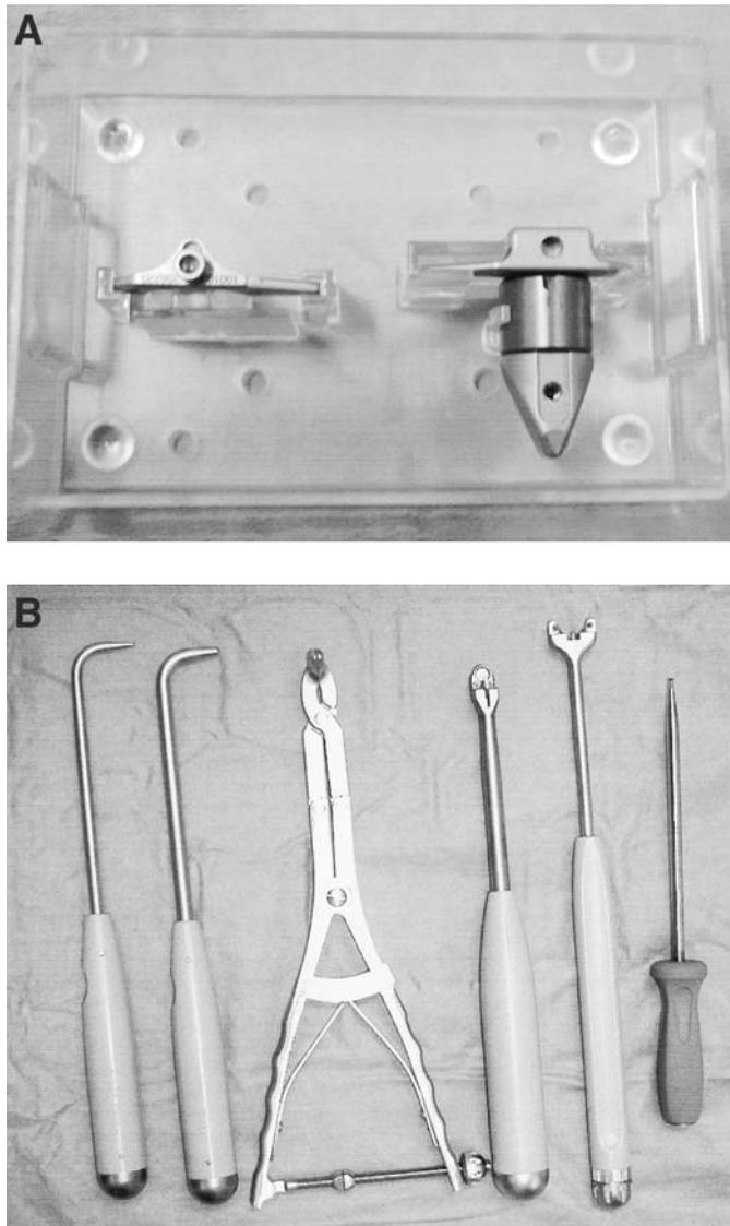
**Fig. 1.** (A) X-Stop device; (B) instrumentation for the device (from left to right): small dilator, intermediate dilator, distraction and measuring instrument, holder for main body of device, holder for wing, torque screwdriver.
