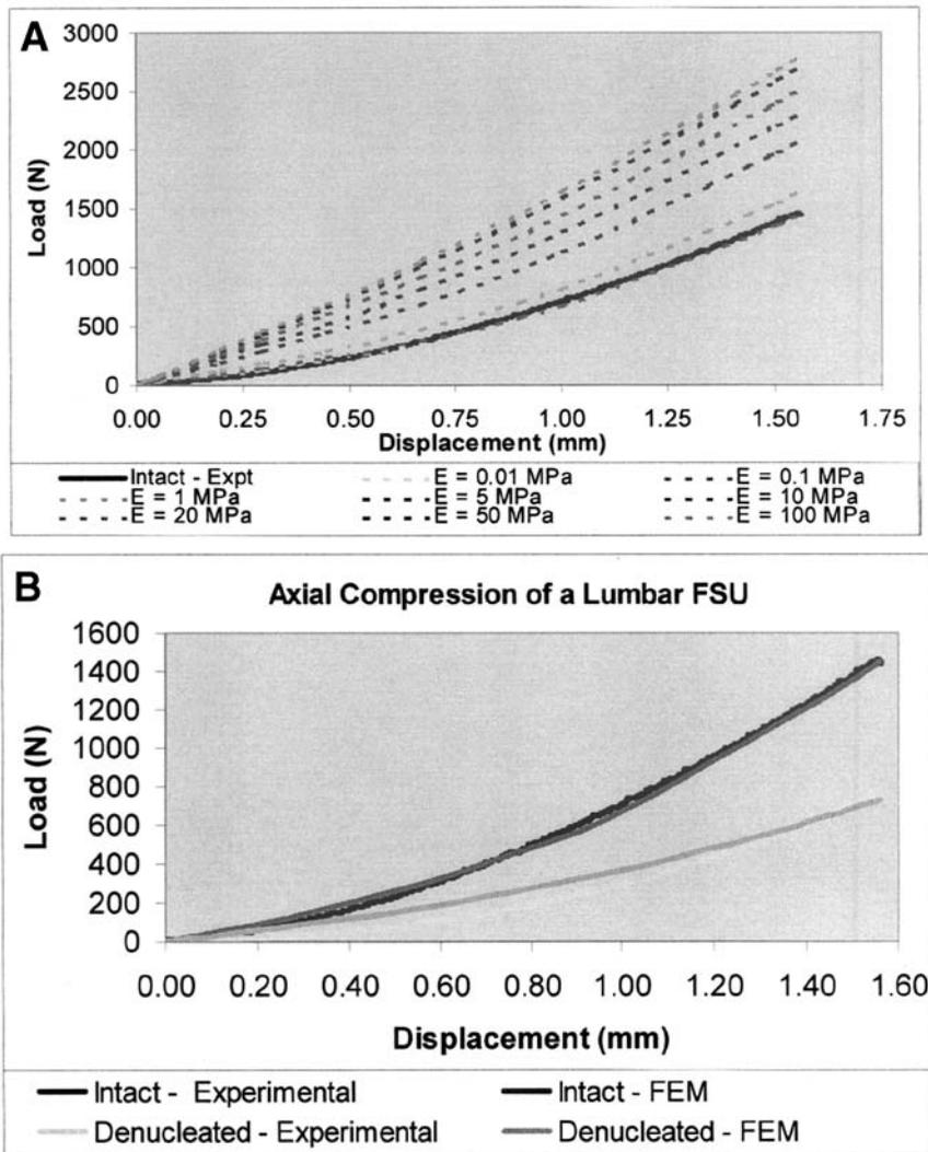
**Fig. 9.** (A) Validation of the FE Model (FEM) to the compressive load-displacement curve of the modeled intact condition to the experimental intact condition. (B) Effect of implant material modulus on load-displacement curves of implanted FSU model. Implant moduli between 0.01 and 1 MPa showed closest matching to the load-displacement curve of the intact experimental FSU.
