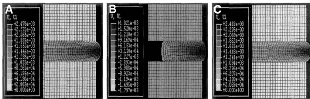
**Fig. 10.** Finite element predictions for radial displacements in (A) intact, (B) denucleated, and (C) PVA/PVP-implanted human lumbar FSU. The radial displacements of the intact and implanted conditions were quite similar, showing tensile displacements in the annulus near the nucleus interface, whereas those of the denucleated condition showed marked differences in that compressive displacements were calculated in the interface between the annulus and the nuclear cavity.
