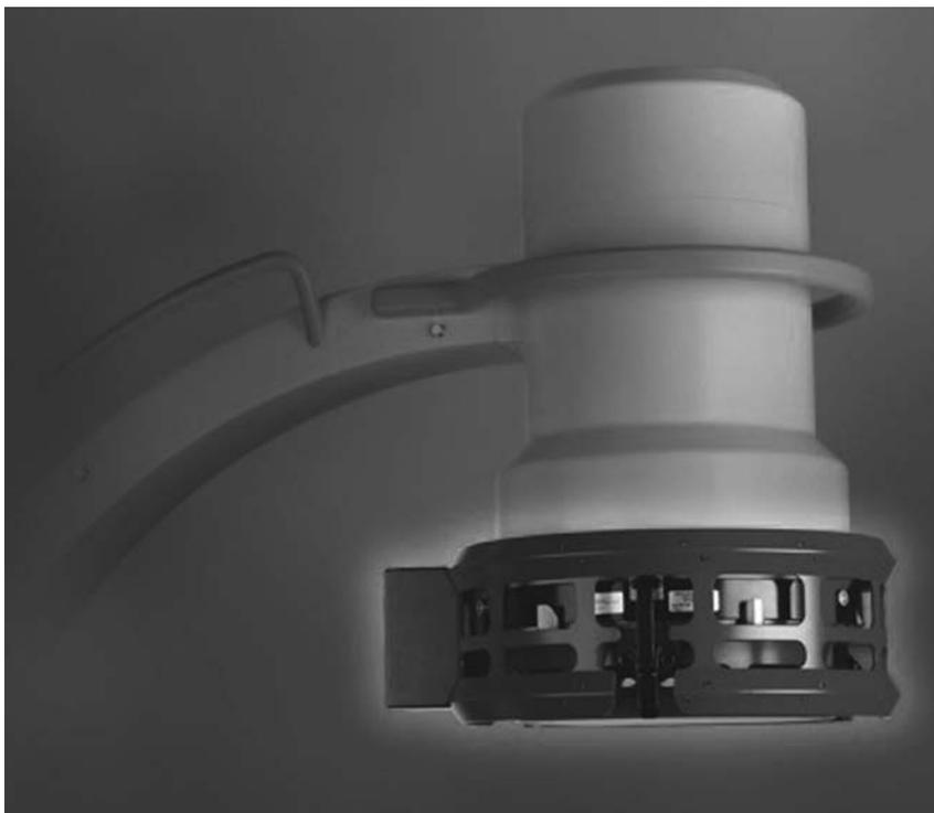
**Fig. 7.** Photograph showing close-up of C-arm with target guide mounted on image intensifier. (Courtesy of Medtronic Sofamor Danek, Memphis, TN.)
