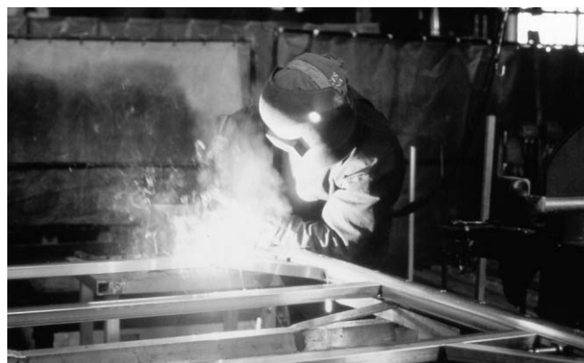
FIGURE 1 Metal Inert Gas (MIG) welding of aluminum.
