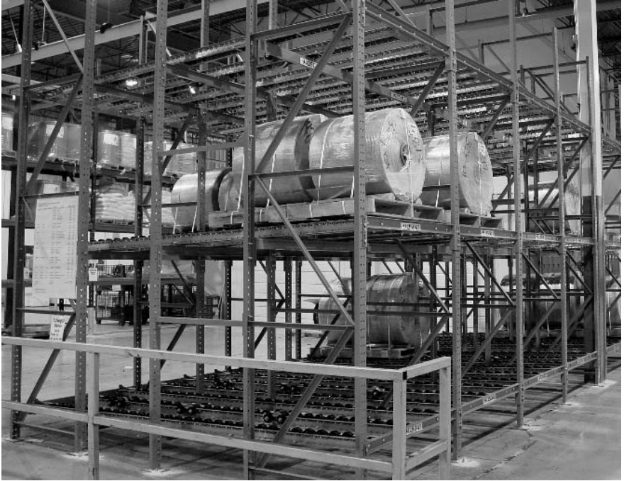
Figure 5-8. Flow racks allow the containers to move forward with use of gravity.
