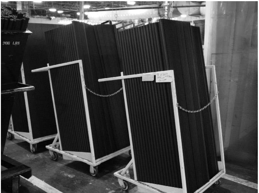
Figure 5-6. Container used as a kanban signal.
