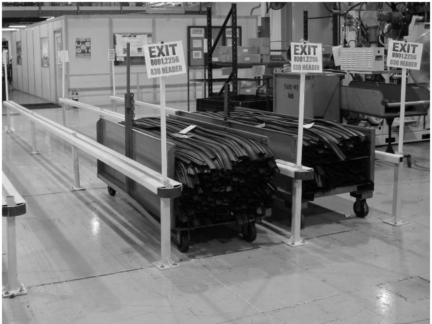
Figure 5-7. Flow lanes with guides to control movement of containers.
