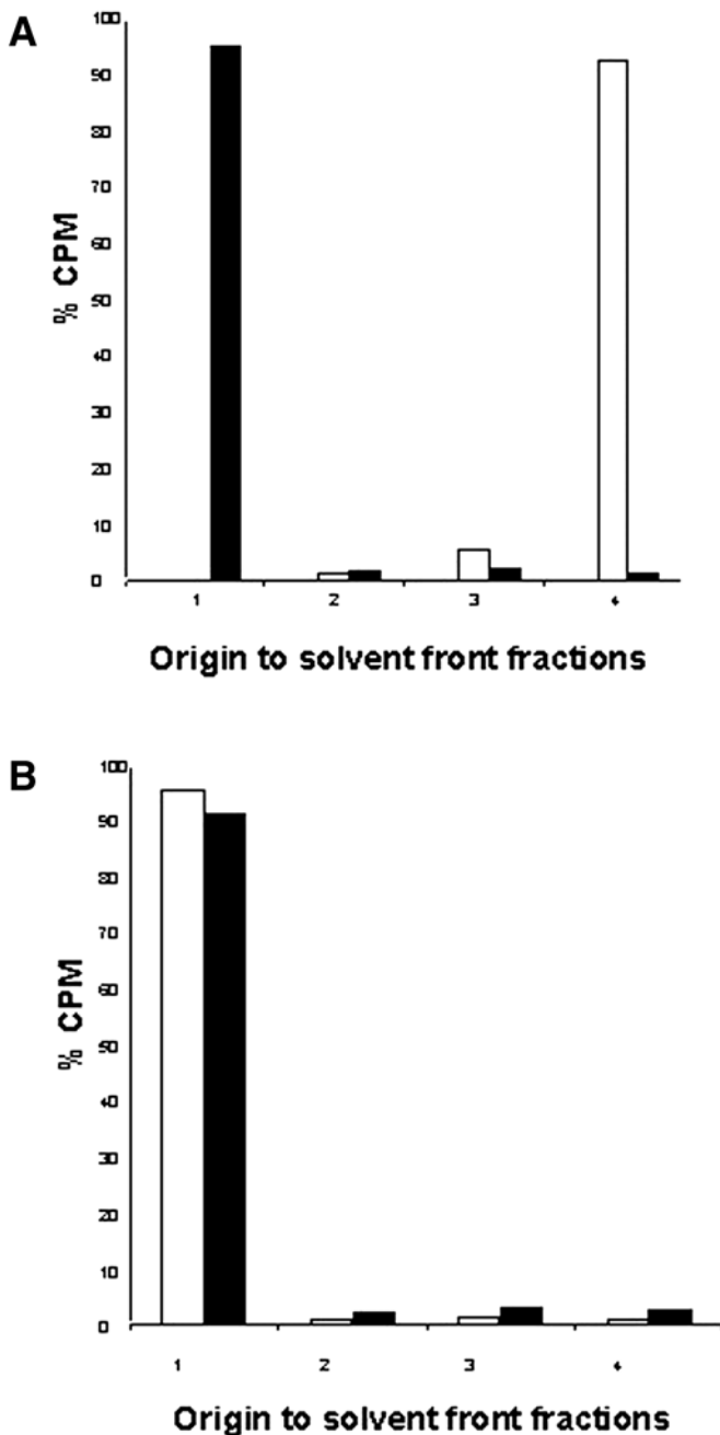
Fig. 2. Analysis of ^{213}\text{Bi} -PAI-2 ( \alpha -PAI-2). (A) Aliquots (10 mL) of freshly eluted \alpha -PAI-2 (filled bars) or ^{213}\text{Bi} standard (unfilled bars) were spotted onto the origin of separate ITLC strips. After mobilization, the strips were cut into four pieces for gamma counting. Fraction 1 corresponds to the sample origin whereas fraction four corresponds to the solvent front. (B) Serum stability of \alpha -PAI-2 incubated at 37^\circ\text{C} in human serum for 0 min (unfilled bars) and 45 min (filled bars) and subjected to ITLC and analyzed as per (A).
