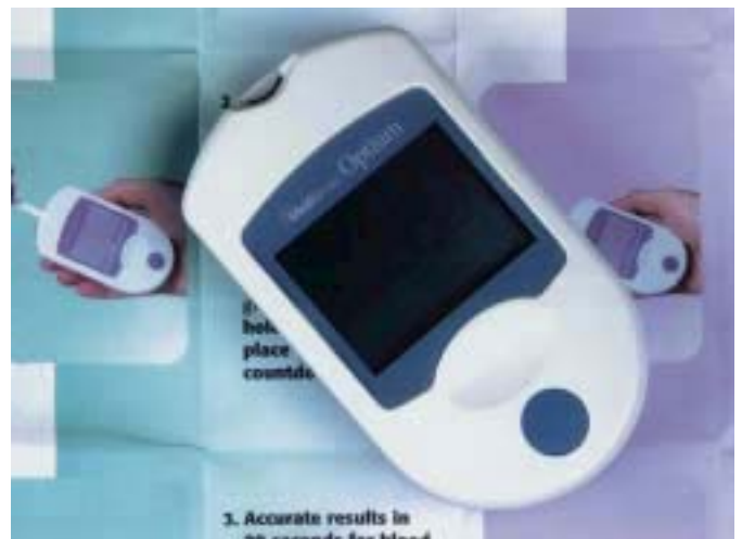
Blood glucose and ketone meter
