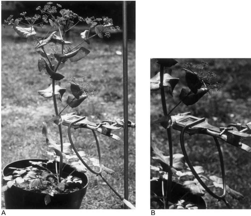
FIGURE 32.13 Simple assimilation chamber for measuring \text{CO}_2 exchange under field conditions.
