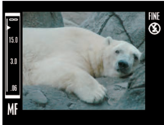
Figure 1-8: On most point-and-shoot cameras, manual focus mode requires you to select a focusing distance from a scale displayed on the monitor.
