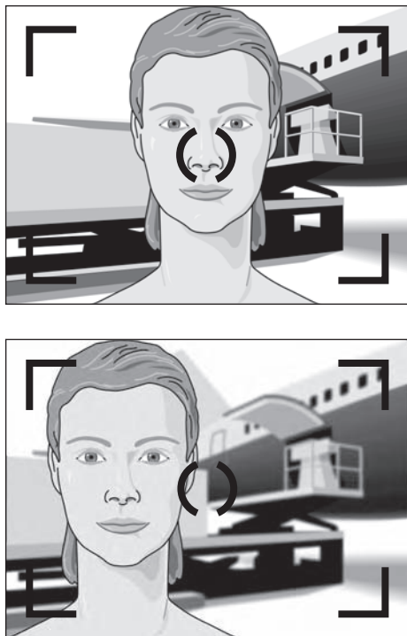
Figure 2-9: After locking the focus and exposure on your main subject, you can reframe the picture before pressing the shutter button the rest of the way down.
