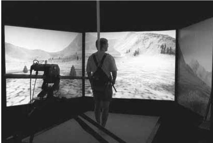
FIGURE 5.3 A typical CAVE installation at the University of Utah. Used by permission. ( http://www.cs.utah.edu/research/areas/immersive/locomotion.html )
