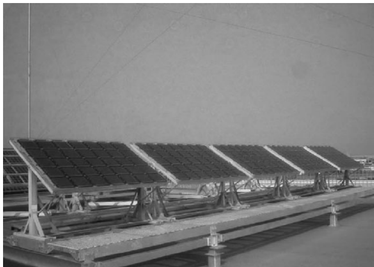
Figure 8.9 Outdoor field tests of DSC modules produced by Aisin Seiki in Kariya City. Note the pc-Si modules in the second row (photograph courtesy of Aisin Seiki).
