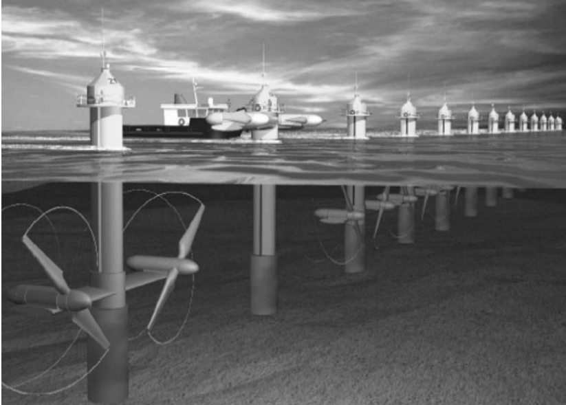
Figure 4.5 Artist's impression of a tidal current turbine farm using horizontal axis turbines (Source: www.marineturbines.com ).
