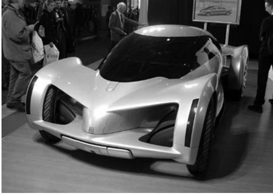
Figure 11.3 General Motors AUTOnomy concept vehicle shows the design possibilities that introduction of fuel cells allows.
