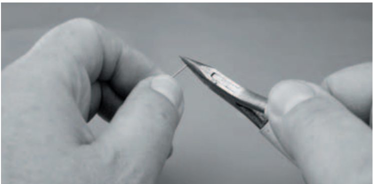
Photo 5.1 Take a short piece of wire between the jaws of your pliers...
