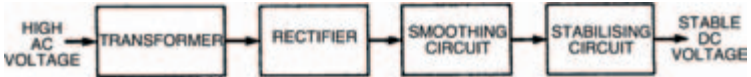
Figure 7.15 A block diagram of a power supply using the circuit stages we have described
