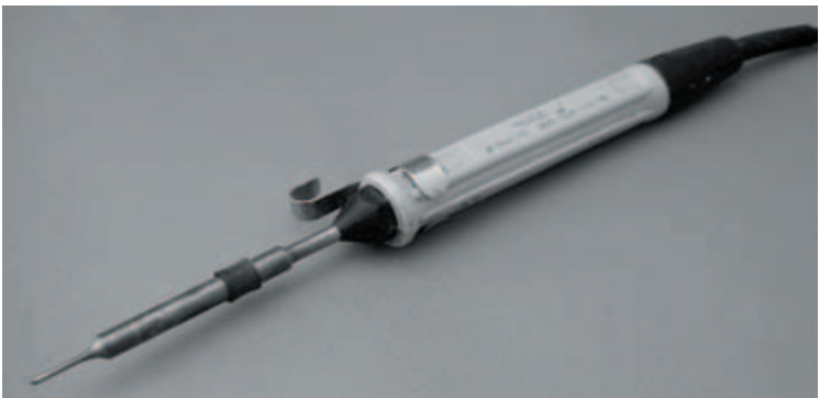
Photo 1.3 Low wattage soldering iron intended for electronics
