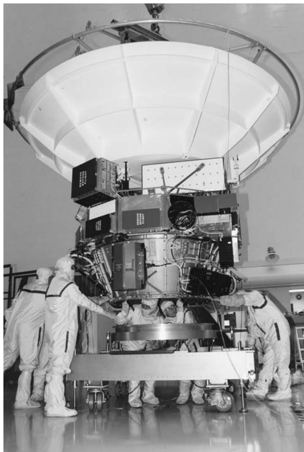
Jet Propulsion Laboratory (JPL) technicians clean and prepare the upper equipment module for mating with the propulsion module of the Cassini orbiter spacecraft at the Kennedy Space Center in 1997. The large Cassini/Huygens spacecraft configuration was successfully launched on October 15, 1997, by a Titan IV-Centaur rocket vehicle. The robot spacecraft arrived at Saturn in July 2004, after a long journey through interplanetary space, which included gravity-assist flybys of Venus (April 1998 and June 1999), Earth (August 1999), and Jupiter (December 2000). (NASA/JPL)
