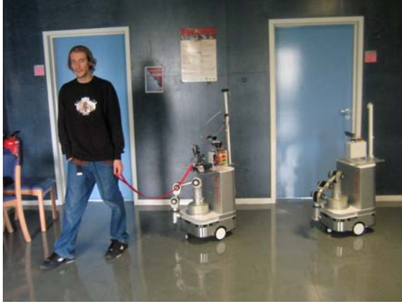
Fig. 6 Example of setup allowing to a human to learn paths to a mobile robot. The control architecture is designed to detect and learn changes in the robot self motor dynamics (strong differences in the proprioceptive flow of the wheels). Thanks to a leash, the human can pull on a sensing device provoking orientation changes of the robot (direct pathway). The robotic arms are not used in this study.
