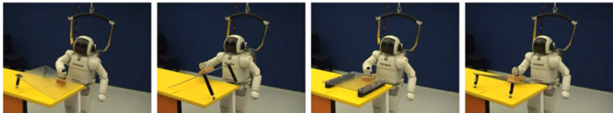
Fig. 14 Reproduced movements on the ASIMO robot for the surface tilted 0^\circ , +16^\circ , -27^\circ about the x -axis, and +16^\circ about the y -axis.
