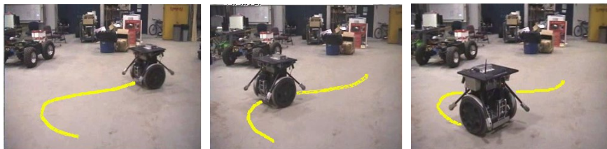
Fig. 3 Segway RMP performing the spatial positioning task (approximate ground path in yellow).
