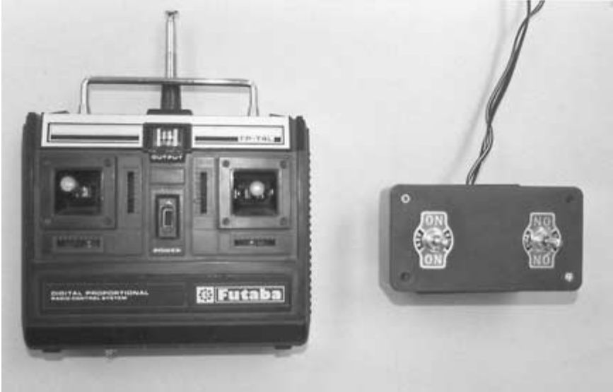
FIGURE I-14. Wireless and wired controls.
