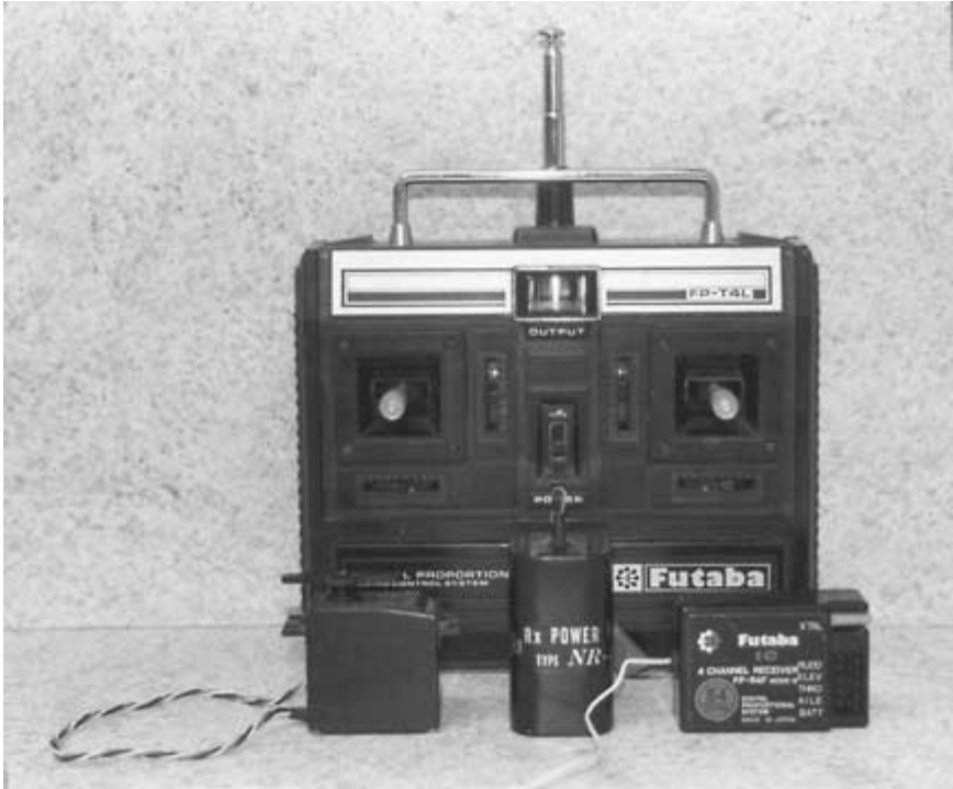
FIGURE 4-1. Three-channel remote control system.
