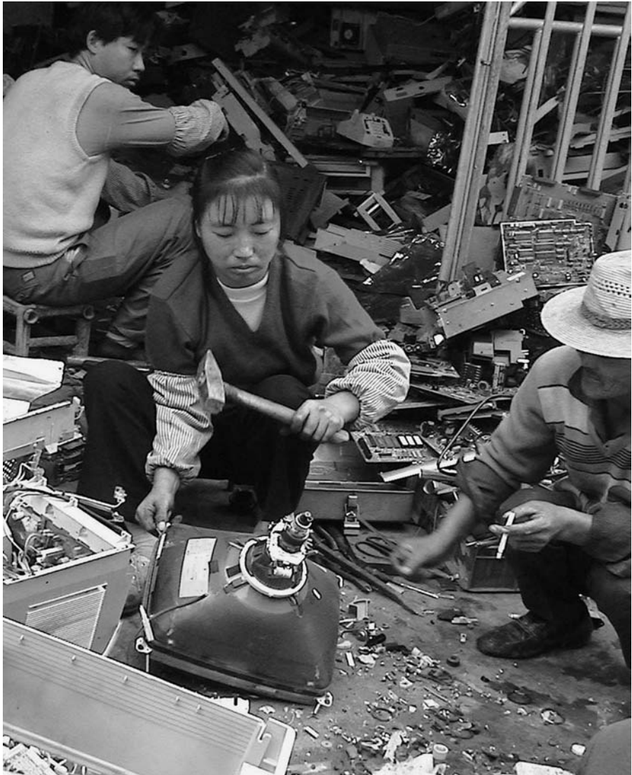
Figure 12.4 Woman prepares to smash a computer monitor cathode-ray tube to recover the copper-containing yoke. Credit: Basel Action Network
