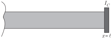
Figure 3.16. Inertially restrained end of a beam
