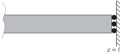
Figure 3.26. Schematic of sliding-end condition
