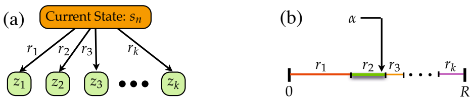
Fig. 4. (a) At step n of the KMC algorithm, the system is in state s_n , and we must choose s_{n+1} from amongst the k possible next states \{z_i\}_{i=1}^k according to their respective transition rates \{r_i\}_{i=1}^k . (b) We can select the next state with a single random number \alpha \sim \text{Uniform}((0, R)) , where R = \sum r_i is the total rate. This example shows the next state chosen to be z_2 .
