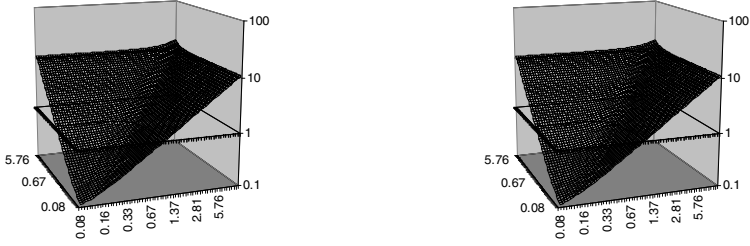
Fig. 4. Norm R = \sqrt{X^2 + Y^2} computed by: (2)–(18) LNS (left); FP (right)
