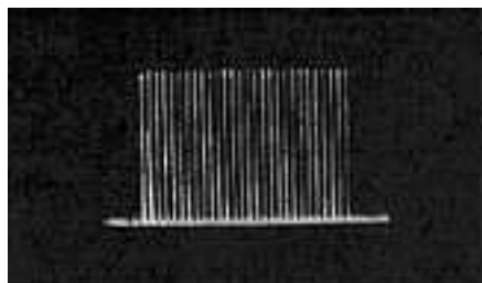
3-8 A spectrum analyzer photo of a Frequency Hop (FH) Spread Spectrum signal.
