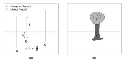
**Figure 22.37.** (a) The *horizon ratio* can be used to determine depth by comparing the visible portion of an object below the horizon to the total vertical visible extent of the object. (b) A real-world example.
