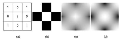
**Figure 11.3.** (a) The image on the left has nine pixels that are all either black or white. The three interpolation strategies are (b) nearest-neighbor, (c) bilinear, and (d) hermite.
