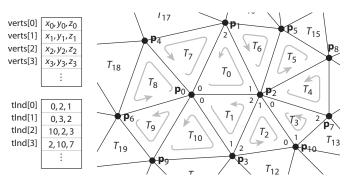
Figure 12.8. A larger triangle mesh, with part of its representation as an indexed triangle mesh.
