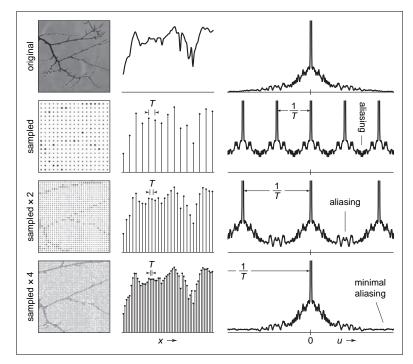
**Figure 9.49.** The effect of sample rate on the frequency spectrum of the sampled signal. Higher sample rates push the copies of the spectrum apart, reducing problems caused by overlap.
