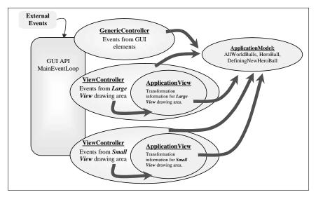
Figure 19.16. Components of the ball shooting program with small view.
