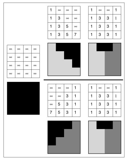
**Figure 8.12.** A z-buffer rasterizing two triangles in each of two possible orders. The first triangle is fully rasterized. The second triangle has every pixel computed, but for three of the pixels the depth-contest is lost, and those pixels are not drawn. The final image is the same regardless.
