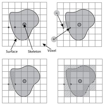
**Figure 16.10.** A section through the cubic lattice. The + sign indicates a vertex inside the surface ( $f(v_i \ge iso)$  and - is outside  $f(v_i < iso)$ .
