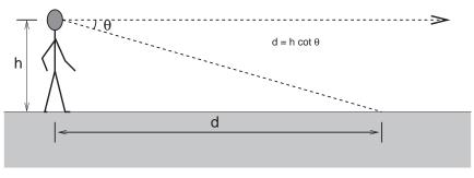
Figure 22.25. Absolute distance to locations on the ground plane can be determined based on declination angle from the horizon and eye height.
