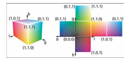
**Plate I.** The RGB color cube in 3D and its faces unfolded. Any RGB color is a point in the cube. (See also Figure 3.13.)
