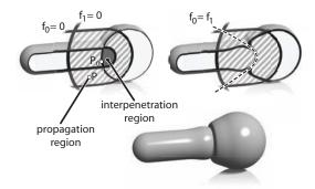
Figure 16.25. A 2D slice through objects in collision showing the various regions and PCM deformation. Image courtesy Erwin DeGroot.
