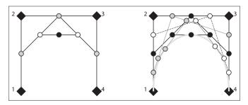
**Figure 15.16.** An illustration of the de Casteljau algorithm for a cubic Bézier. The left-hand image shows the construction for u = 0.5. The right-hand image shows the construction for 0.25, 0.5, and 0.75.
