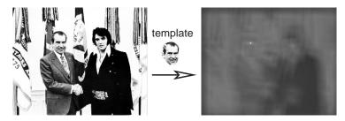
**Figure 22.34.** Template matching. The bright spot in the right image indicates the best match location to the template in the left image. *Image courtesy National Archives and Records Administration.*
