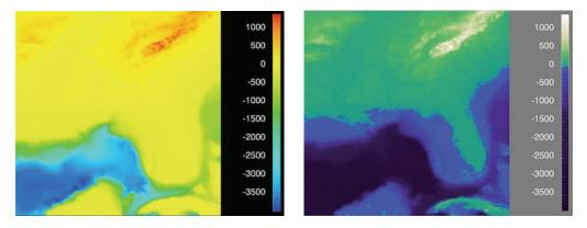
**Plate XLIV.** Left: The standard rainbow colormap has two defects: it uses hue to denote ordering, and it is not perceptually isolinear. (See also Figure 27.8.) Right: The structure of the same dataset is far more clear with a colormap where monotonically increasing lightness is used to show ordering and hue is used instead for segmenting into categorical regions. (See also Figure 27.9.) *Courtesy Bernice Rogowitz.*
