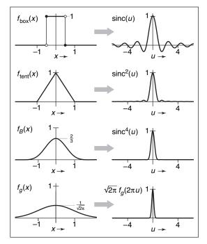
Figure 9.46. The Fourier transforms of the box, tent, B-spline, and Gaussian filters.
