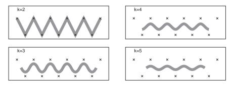
**Figure 15.1.** B-spline curves using the same uniform set of knots and the same control points, for various values of *k*. Note that as *k* increases, the valid parameter range for the curve shrinks.
