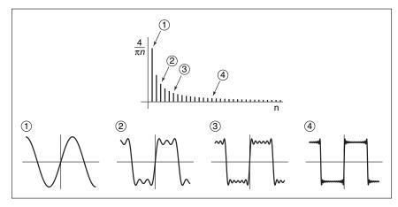
Figure 9.41. Approximating a square wave with finite sums of sines.
