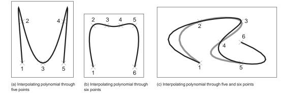
**Figure 15.3.** Interpolating polynomials through multiple points. Notice the extra wiggles and over-shooting between points. In (c), when the sixth point is added, it completely changes the shape of the curve due to the non-local nature of interpolating polynomials.
