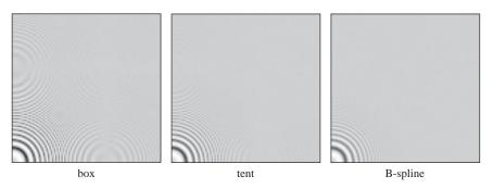
**Figure 9.35.** A comparison of three different sampling filters being used to antialias a difficult test image that contains circles that are spaced closer and closer as they get larger.
