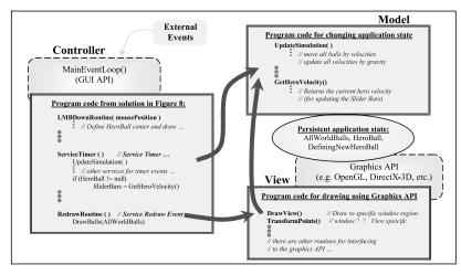
Figure 19.10. Components of an interactive graphics application.
