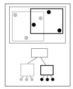
**Figure 12.27.** The gray box is a tree node that points to the three gray spheres, and the thick black box points to the three black spheres. Note that not all spheres enclosed by the box are guaranteed to be pointed to by the corresponding tree node.
