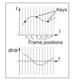
**Figure 17.5.** A continuous curve f(t) is fit through the keys provided by the animator even though only values at frame positions are of interest. The derivative of this function gives the speed of parameter change and is at first determined automatically by the fitting procedure.
