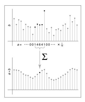
**Figure 9.4.** Computing one value in the discrete convolution of a sequence *b* with a filter *a* that has support five samples wide. Each sample in  $a \star b$  is an average of nearby samples in *b*, weighted by the values of *a*.
