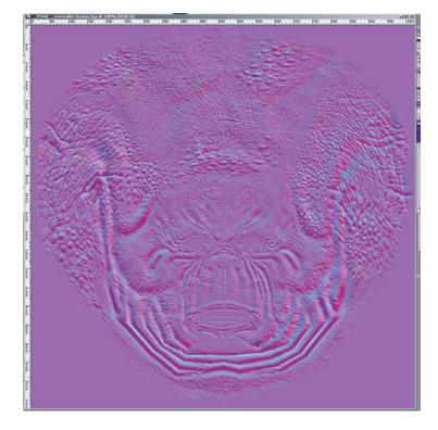
**Plate XXXVI.** The normal map used in Figure 26.8. In this image, the red, green and blue channels of the texture contain the X, Y, and Z coordinates of the surface normals. *Image courtesy Keith Bruns.* (See also Figure 26.9.)
