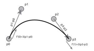
**Figure 15.10.** A cubic Bézier curve is controlled by four points. It interpolates the first and last, and the beginning and final derivatives are three times the vectors between the first two (or last two) points.
