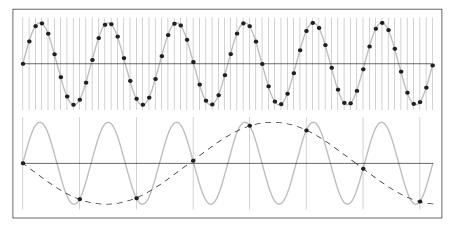
**Figure 9.2.** A sine wave (gray curve) sampled at two different rates. Top: at a high sample rate, the resulting samples (black dots) represent the signal well. Bottom: a lower sample rate produces an ambiguous result: the samples are exactly the same as would result from sampling a wave of much lower frequency (dashed curve).
