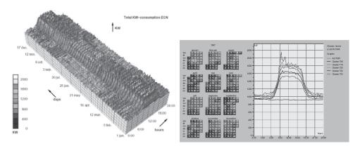
**Figure 27.10.** Left: A 3D representation of this time series dataset introduces the problems of occlusion and perspective distortion. Right: The linked 2D views of derived aggregate curves and the calendar allow direct comparison and show more fine-grained patterns. *Image courtesy Jarke van Wijk* (van Wijk & van Selow, 1999), © 1999 IEEE. (See also Plate XLV.)
