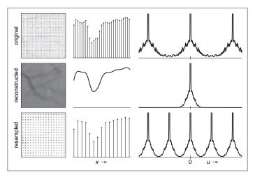
**Figure 9.53.** Resampling viewed in the frequency domain. The resampling filter both reconstructs the signal (removes the alias spectra) and bandlimits it (reduces its width) for sampling at the new rate.
