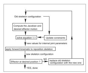
Figure 17.19. A diagram of the inverse kinematic algorithm.
