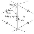
Figure 12.18. The references from a half-edge to its neighboring mesh components.
