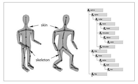
**Figure 17.15.** (Left) A hierarchy of joints, a skeleton, serves as a kinematic abstraction of the character; (middle) repositioning the skeleton deforms a separate skin object attached to it; (right) a tree data structure is used to represent the skeleton. For compactness, the internal structure of several nodes is hidden (they are identical to a corresponding sibling).
