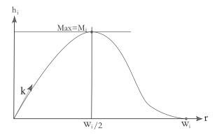
**Figure 16.26.** The function,  $h_i(r)$  is the value of the deformation function  $w_i$  in the propagation region.
