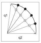
Figure 17.12. Interpolating quaternions should be done on the surface of a 3D unit sphere embedded in 4D space. However, much simpler interpolation along a 4D straight line (open circles) followed by re-projection of the results onto the sphere (black circles) is often sufficient.
