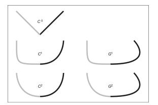
Figure 15.2. An illustration of various types of continuity between two curve segments.
