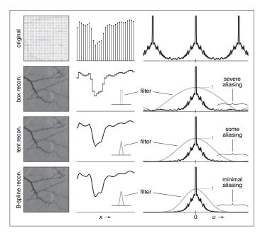
**Figure 9.52.** The effects of different reconstruction filters in the frequency domain. A good reconstruction filter attenuates the alias spectra effectively while preserving the base spectrum.
