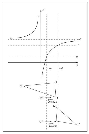
**Figure 8.7.** The depth *z* is transformed to the depth z' by the perspective transform. Note that when *z* moves from positive to negative, z' switches from negative to positive. Thus vertices behind the eye are moved in front of the eye beyond z' = n + f. This will lead to wrong results, which is why the triangle is first clipped to ensure all vertices are in front of the eye.
