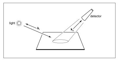
**Figure 20.5.** A simple measurement device for directional reflectance. The positions of light and detector are moved to each possible pair of directions. Note that both  $\mathbf{k}_i$  and  $\mathbf{k}_o$  point away from the surface to allow reciprocity.
