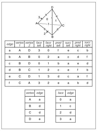
**Figure 12.15.** A tetrahedron and the associated elements for a winged-edge data structure. The two small tables are not unique; each vertex and face stores any one of the edges with which it is associated.
