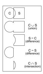
Figure 13.6. The basic CSG operations on a 2D circle and square.
