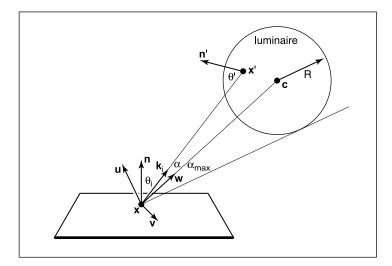
Figure 24.7. Geometry for direct lighting at point x from a spherical luminaire.
