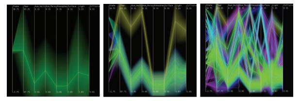
Plate LI. Hierarchical parallel coordinates show high-dimensional data at multiple levels of detail. *Image courtesy Matt Ward* (Fua et al., 1999), © 1999 IEEE. (See also Figure 27.21).
