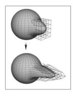
**Figure 17.14.** Adjusting the FFD lattice results in the deformation of the object.
