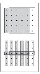
Figure 9.30. Computing two output points using separate 2D arrays of 25 samples (above) vs. filtering once along the columns, then using separate 1D arrays of five samples (below).
