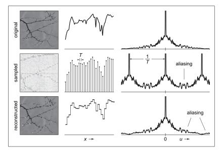
**Figure 9.48.** Sampling and reconstruction with no filtering. Sampling produces alias spectra that overlap and mix with the base spectrum. Reconstruction with a box filter collects even more information from the alias spectra. The result is a signal that has serious aliasing artifacts.
