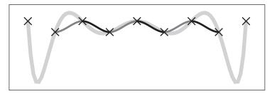
**Figure 15.9.** Splines interpolating nine control points (marked with small crosses). The thick gray line shows an interpolating polynomial. The thin, dark line shows a Catmull-Rom spline. The latter is made of seven cubic segments, which are each shown in alternating gray tones.
