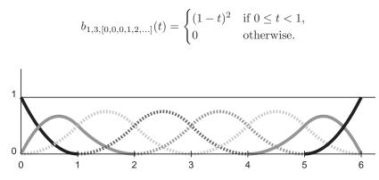
**Figure 15.24.** Endpoint-interpolating quadratic (k = 3) B-splines, for n = 8. The knot vector is [0,0,0,1,2,3,4,5,6,6,6]. The first and last two B-splines are aperiodic, while the middle four (shown as dotted lines) are periodic and identical to the ones in Figure 15.20.
