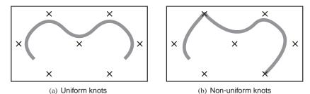
**Figure 15.23.** A curve parameterized by quadratic B-splines (k = 3) with seven control points. On the left, uniform knots vector [1,2,3,4,5,6,7,8,9,10] is used. On the right, the non-uniform knot spacing [1,2,3,4,4,6,7,8,8,10] is used. The duplication of the 4th and 8th knot means that all interior knots of the 3rd and 7th B-spline are equal, so the curve interpolates the control point associated with those points.
