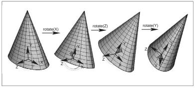
**Figure 17.10.** Three Euler angles can be used to specify arbitrary object orientation through a sequence of three rotations around coordinate axes embedded into the object (axis Y always points to the tip of the cone). Note that each rotation is given in a new coordinate system. Fixed angle representation is very similar but the coordinate axes it uses are fixed in space and do not rotate with the object.
