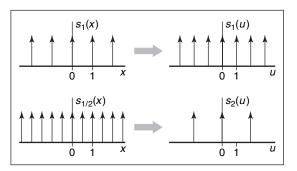
**Figure 9.47.** Impulse trains. The Fourier transform of an impulse train is another impulse train. Changing the period of the impulse train in space causes an inverse change in the period in frequency.
