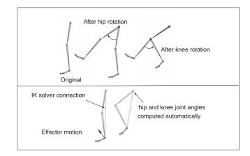
**Figure 17.16.** Forward kinematics (top) requires the animator to put all joints into correct position. In inverse kinematic (bottom), parameters of some internal joints are computed based on desired end effector motion.
