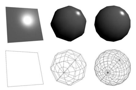
**Figure 18.8.** The results of running the fragment shader from Section 18.3.4. Note that the Phong highlight does appear on the left-most model which is represented by a single polygon. In fact, because lighting is calculated at the fragment, rather than at each vertex, the more coarsely tessellated sphere models also demonstrate appropriate Phong shading. (See also Plate IX.)
