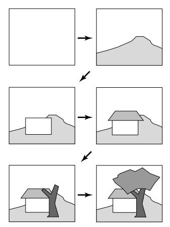
Figure 12.33. A painter's algorithm starts with a blank image and then draws the scene one object at a time from back-to-front, overdrawing whatever is already there. This automatically eliminates hidden surfaces.
