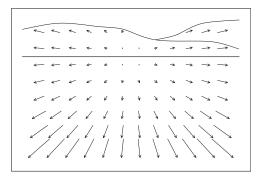
**Figure 22.41.** The optic flow generated by moving through an otherwise static environment provides information about both the motion relative to the environment and the distances to points in the environment. In this case, the direction of view is depressed from the horizon, but as indicated by the focus of expansion, the motion is parallel to the ground plane.
