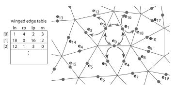
Figure 12.14. An example of a winged-edge mesh structure, stored in arrays.
