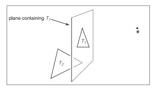
**Figure 12.35.** When **e** and  $T_2$  are on opposite sides of the plane containing  $T_1$ , then it is safe to draw  $T_2$  first and  $T_1$  second. If **e** and  $T_2$  are on the same side of the plane, then  $T_1$  should be drawn before  $T_2$ . This is the core idea of the BSP tree algorithm.
