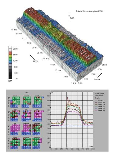
Plate XLV. Top: A 3D representation of this time series dataset introduces the problems of occlusion and perspective distortion. Bottom: The linked 2D views of derived aggregate curves and the calendar allow direct comparison and show more fine-grained patterns. *Image courtesy Jarke van Wijk* (van Wijk & van Selow, 1999), © 1999 IEEE. (See also Figure 27.10.)
