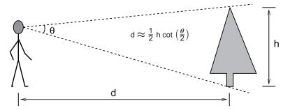
**Figure 22.36.** The *size-distance relationship* allows the distance to objects of known size to be determined based on the visual angle subtended by the object. Likewise, the size of an object at a know distance can be determined based on the visual angle subtended by the object.
