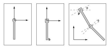
**Figure 12.19.** A hinged pendulum. On the left are the two pieces in their "local" coordinate systems. The hinge of the bottom piece is at point **b** and the attachment for the bottom piece is at its local origin. The degrees of freedom for the assembled object are the angles  $(\theta, \phi)$  and the location **p** of the top hinge.
