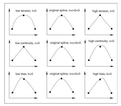
**Figure 17.6.** Editing the default interpolating spline (middle column) using TCB controls. Note that all keys remain at the same positions.
