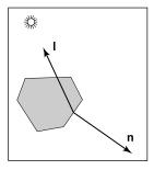
Figure 10.2. When a surface points away from the light, it should receive no light. This case can be verified by checking whether the dot product of I and n is negative.
