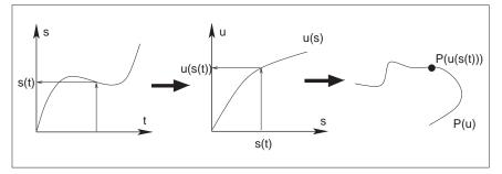
**Figure 17.8.** To get position in space at a given time *t*, one first utilizes user-specified motion control to obtain the distance along the curve s(t) and then compute the corresponding curve parameter value u(s(t)). Previously fitted curve P(u) can now be used to find the position P(u(s(t))).
