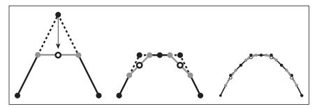
**Figure 15.14.** Subdivision procedure for quadratic Béziers. Each line segment is divided in half and these midpoints are connected (gray points and lines). The interior control point is moved to the midpoint of the new line segment (white circle).
