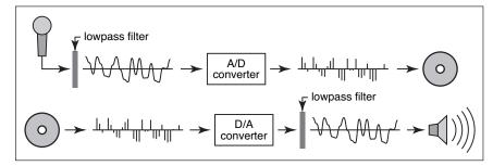
Figure 9.1. Sampling and reconstruction in digital audio.
