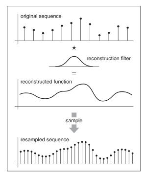
**Figure 9.36.** Resampling an image consists of two logical steps that are combined into a single operation in code. First, we use a reconstruction filter to define a smooth, continuous function from the input samples. Then, we sample that function on a new grid to get the output samples.
