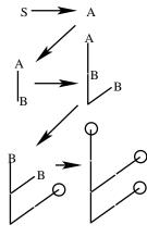
Figure 17.27. Consecutive derivation steps using a simple L-system. Capital letters denote non-terminals and illustrate positions at which corresponding non-terminal will be expanded. They are not part of the actual output.
