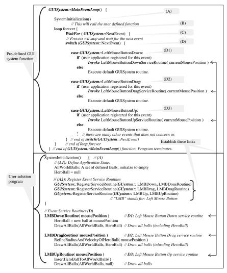
Figure 19.7. Linking MainEventLoop with our solution.
