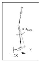
**Figure 17.17.** Partial derivative  $\partial x / \partial \alpha_{\text{knee}}$  is given by the limit of  $\Delta x / \Delta \alpha_{\text{knee}}$ . Effector displacement is computed while all joints, except the knee, are kept fixed.
