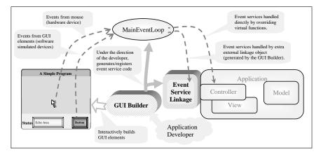
Figure 19.18. Working with a GUI API.
