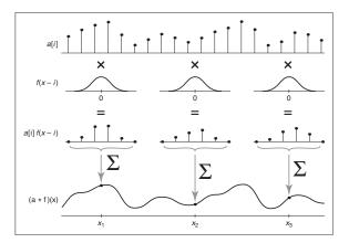
Figure 9.14. Discrete-continuous convolution.
