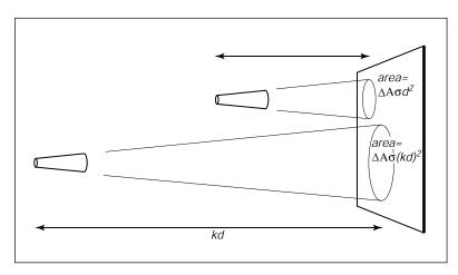
**Figure 20.2.** The signal a radiance detector receives does not depend on the distance to the surface being measured. This figure assumes the detectors are pointing at areas on the surface that are emitting light in the same way.
