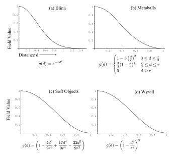
**Figure 16.2.** Fall-off filter functions ( $0 \le r \le 1$ ). (a) Blinn's Gaussian or "blobby" function; (b) Nishimura's "metaball" function; (c) Wyvill et al.'s "soft objects" function; (d) the Wyvill function.
