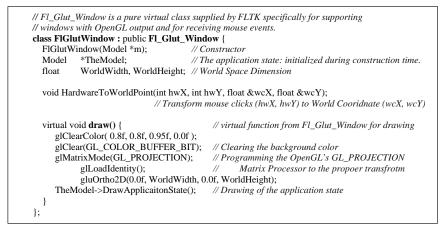
Figure 19.23. FIGlutWindow: OpenGL/FLTK view/controller pair.
