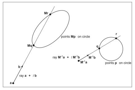
**Figure 13.5.** The ray intersection problem in the two spaces are just simple transforms of each other. The object is specified as a sphere plus matrix  $\mathbf{M}$ . The ray is specified in the transformed (world) space by location  $\mathbf{a}$  and direction  $\mathbf{b}$ .
