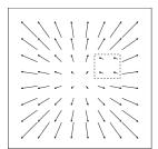
**Figure 22.42.** Visual detection of moving objects from a moving observation point requires recognizing patterns in the optic flow that cannot be associated with motion through a static environment.
