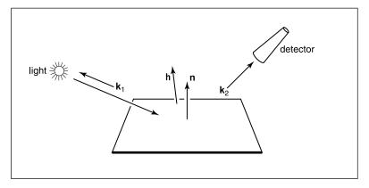
Figure 25.6. Geometry of reflection. Note that  $k_1$ ,  $k_2$ , and h share a plane, which usually does not include n.
