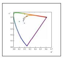
**Plate XXXI.** A series of light sources plotted in the CIE u'v' chromaticity diagram. A white piece of paper illuminated by any of these light sources maintains a white color appearance. (See also Figure 21.11.)
