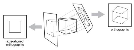
**Figure 4.3.** When projection lines are parallel and perpendicular to the image plane, the resulting views are called orthographic.
