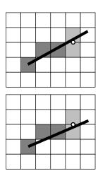
Figure 8.3. Top: the line goes above the midpoint so the top pixel is drawn. Bottom: the line goes below the midpoint so the bottom pixel is drawn.
