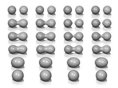
Figure 16.3. Each column shows two point primitives approaching each other. From left to right: the fall-off filter functions used are Blobby, Metaball, soft objects, and Wyvill. *Image courtesy Erwin DeGroot*.
