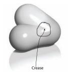
Figure 16.19. Two point primitives on the left are connected by the Ricci union. A third primitive is blended to the result, creating an unwanted crease in the field. *Image courtesy Erwin DeGroot*.
