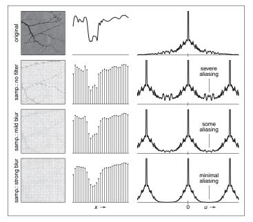
**Figure 9.51.** How the lowpass filters from Figure 9.50 prevent aliasing during sampling. Lowpass filtering narrows the spectrum so that the copies overlap less, and the high frequencies from the alias spectra interfere less with the base spectrum.
