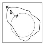
Figure 11.13. The points **p** on the circle are each displaced in the direction of **n** by the function  $f(\mathbf{p})$ . If *f* is continuous, then the resulting points  $\mathbf{p}'$  form a continuous surface.
