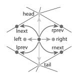
**Figure 12.16.** The references from an edge to the neighboring edges, faces, and vertices in the winged-edge structure.
