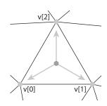
**Figure 12.7.** The triangleto-vertex references in a shared-vertex mesh.
