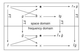
**Figure 9.45.** A commutative diagram to show visually the relationship between convolution and multiplication. If we multiply f and g in space, then transform to frequency, we end up in the same place as if we transformed f and g to frequency and then convolved them. Likewise, if we convolve f and g in space and then transform into frequency, we end up in the same place as if we transformed f and g to frequency, then multiplied them.
