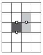
**Figure 8.4.** When using the decision point shown between the two light gray pixels, we just drew the dark gray pixel, so we evaluated *f* at one of the two left points shown.
