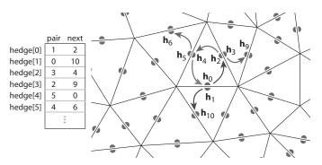
Figure 12.17. An example of a half-edge mesh structure, stored in arrays.
