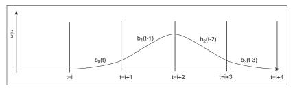
**Figure 15.22.** The cubic (k = 4) B-spline with uniform knots.
