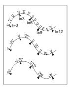
**Figure 17.7.** All three motions are along the same 2D path and satisfy the set of keys at the tips of the black triangles. The tips of the white triangles show object position at  $\Delta t = 1$  intervals. Uniform speed of motion between the keys (top) might be closer to what the animator wanted but automatic fitting procedures could result in either of the other two motions.
