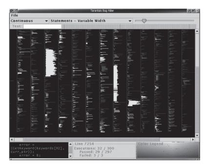
**Figure 27.11.** Tarantula shows an overview of source code using one-pixel lines color coded by execution status of a software test suite. *Image courtesy John Stasko* (Jones et al., 2002). (See also Plate XLVI.)
