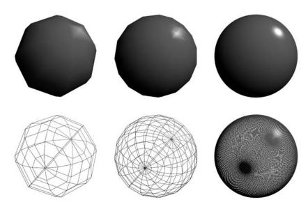
**Figure 18.7.** Each sphere is rendered using only a vertex shader that computes Phong shading. Because the computation is being performed on a per-vertex basis, the Phong highlight only begins to appear accurate after the amount of geometry used to model the sphere is increased drastically. (See also Plate VIII.)
