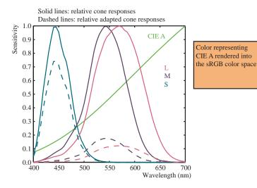
**Plate XXXII.** An example of von Kries–style independent photoreceptor gain control. The relative cone responses (solid line) and the relative adapted cone responses to CIE illuminant A (dashed) are shown. The separate patch of color represents CIE illuminant A rendered into the sRGB color space. (See also Figure 21.12.)
