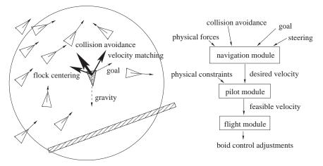
**Figure 17.28.** (Left) Individual flock member (boid) can experience several urges of different importance (shown by line thickness) which have to be negotiated into a single velocity vector. A boid is aware of only its limited neighborhood (circle). (Right) Boid control is commonly implemented as three separate modules.
