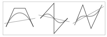
**Figure 15.12.** The *variation diminishing* property of Bézier curves means that the curve does not cross a line more than its control polygon does. Therefore, if the control polygon has no "wiggles," the curve will not have them either. B-splines (Section 15.6.2) also have this property.
