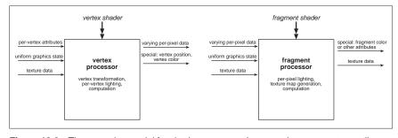
**Figure 18.6.** The execution model for shader programs. Input, such as per-vertex attributes, graphics state-related uniform variables, varying data, and texture maps are provided to vertex and fragment programs within the shader processor. Shaders output special variables used in later parts of the graphics pipeline.
