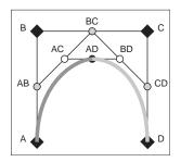
**Figure 15.17.** The de Casteljau algorithm is used to subdivide a cubic Bézier segment. The initial points (black diamonds A, B, C, and D) are linearly interpolated to yield gray circles (AB, BC, CD), which are linearly interpolated to yield white circles (AC, BD), which are linearly interpolated to give the point on the cubic AD. This process also has subdivided the Bézier segment with control points A, B, C, D into two Bézier segments with control points A, AB, AC, AD and AD, BD, CD, D.
