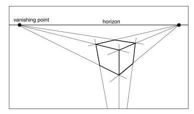
**Figure 4.5.** In three-point perspective, an artist picks "vanishing points" where parallel lines meet. Parallel horizontal lines will meet at a point on the horizon. Every set of parallel lines has its own vanishing points. These rules are followed automatically if we implement perspective based on the correct geometric principles.
