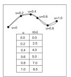
Figure 17.9. To create a tabular version of s(u), the curve can be approximated by a number of line segments connecting points on the curve positioned at equal parameter increments. The table is searched to find the uinterval for a given S. For the curve above, for example, the value of u corresponding to the position of S = 6.5 lies between u = 0.6and *u* = 0.8.
