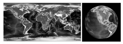
**Figure 11.8.** A Miller cylindrical projection map world map and its placement on the sphere. The distortions in the texture map (i.e., Greenland being so large) exactly correspond to the shrinking that occurs when the map is applied to the sphere.
