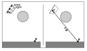
**Figure 13.13.** Left: an area light can be approximated by some number of point lights; four of the nine points are visible to **p** so it is in the penumbra. Right: a random point on the light is chosen for the shadow ray, and it has some chance of hitting the light or not.
