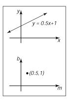
**Figure 14.3.** The set of points on the line y = mx + b in (x, y) space can also be represented by a single point in (m, b) space so the top line and the bottom point represent the same geometric entity: a 2D line.
