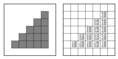
Figure 8.5. A colored triangle with barycentric interpolation. Note that the changes in color components are linear in each row and column as well as along each edge. In fact it is constant along every line, such as the diagonals, as well. (See also Plate II.)
