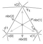
**Figure 12.12.** The references between triangles and vertices in the triangle neighbor structure.
