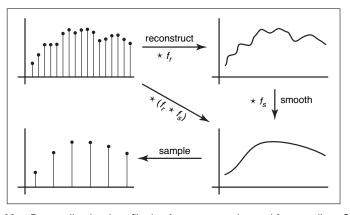
**Figure 9.38.** Resampling involves filtering for reconstruction and for sampling. Since two convolution filters applied in sequence can be replaced with a single filter, we only need one resampling filter, which serves the roles of reconstruction and sampling.
