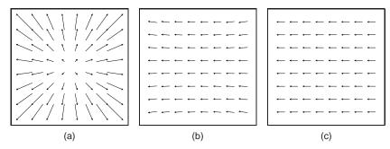
**Figure 22.40.** (a) Movement towards a flat, textured surface produces an expanding flow field, with the *focus of expansion* indicating the line of sight corresponding to the direction of motion. (b) The flow field resulting from rotation around the vertical axis while viewing a flat surface oriented perpendicularly to the line of sight. (c) The flow field resulting from translation parallel to a flat, textured surface.
