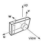
Figure 4.8. The vectors of the camera frame, together with the view direction and up direction. The  $\mathbf{w}$  vector is opposite the view direction, and the  $\mathbf{v}$  vector is coplanar with  $\mathbf{w}$  and the up vector.
