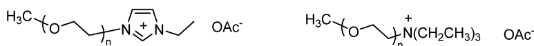
Scheme 5.5. Imidazolium- and ammonium-based ILs consisting of alkyloxyalkyl-substituted cation and acetate anion (abbreviated as [Me(OEt) n -Et-Im][OAc] and [Me(OEt) n -Et 3 N][OAc] respectively) ( n = 2, 3, \dots ).
