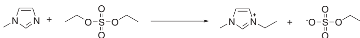
Figure 3.17. Halide-free synthesis route for the preparation of [EMIM][EtSO 4 ] with diethyl sulfate as alkylating agent.
