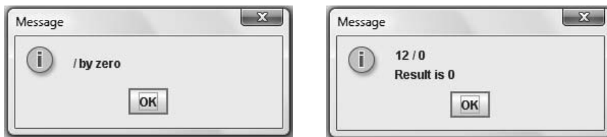
Figure 11-40 Output of the PerformDivision application when the user enters 12 and 0
