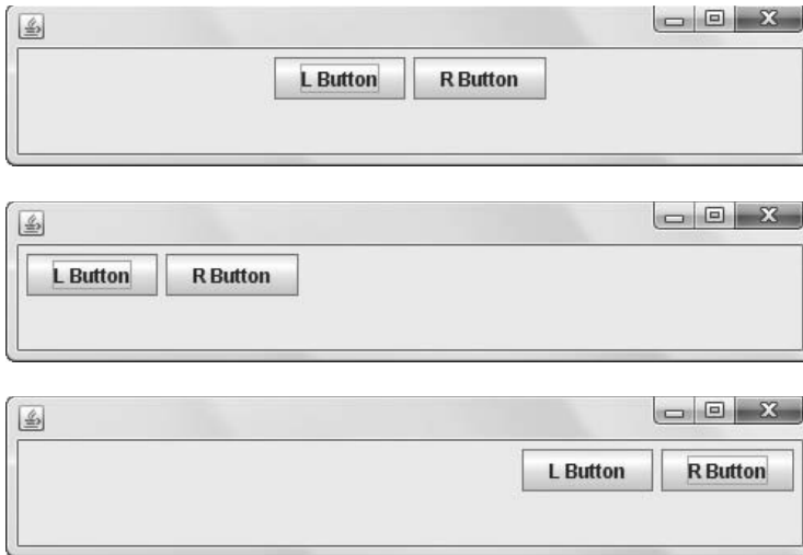
Figure 14-13 The JDemoFlowLayout application as it first appears on the screen, after the user chooses the “L” button, and after the user chooses the “R” button
