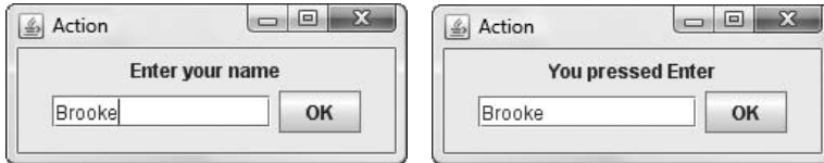
Figure 13-39 Typical execution of the JAction2 application
