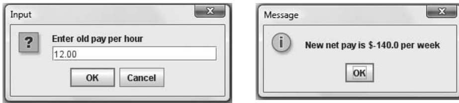
Figure 11-34 Input and incorrect output produced by PayRaise application in Figure 11-33
