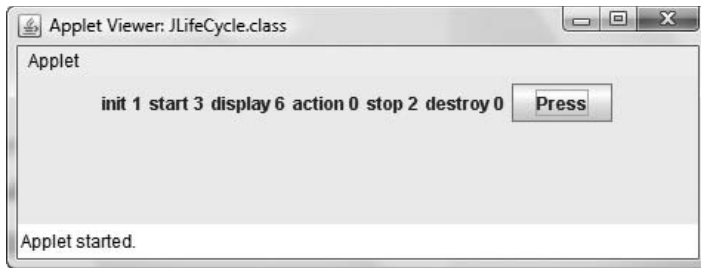
Figure 16-18 The JLifeCycle JApplet after minimizing and restoring twice
