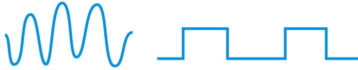
Figure 3.2 An analog and a digital signal
