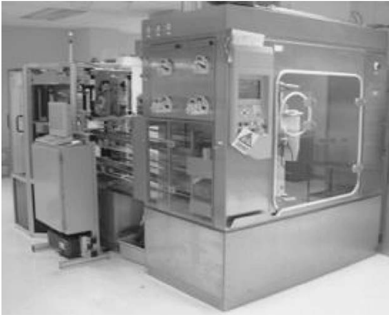
FIGURE 2 Photograph of the Cellmate™ robot built by The Technology Partnership, Cambridge, U.K. This robot performs cell seeding in either large T flasks or roller bottles, exchanges media, rinses cell sheets, purges gases, harvests cells by trypsinization or scraping, and supports transfections.
