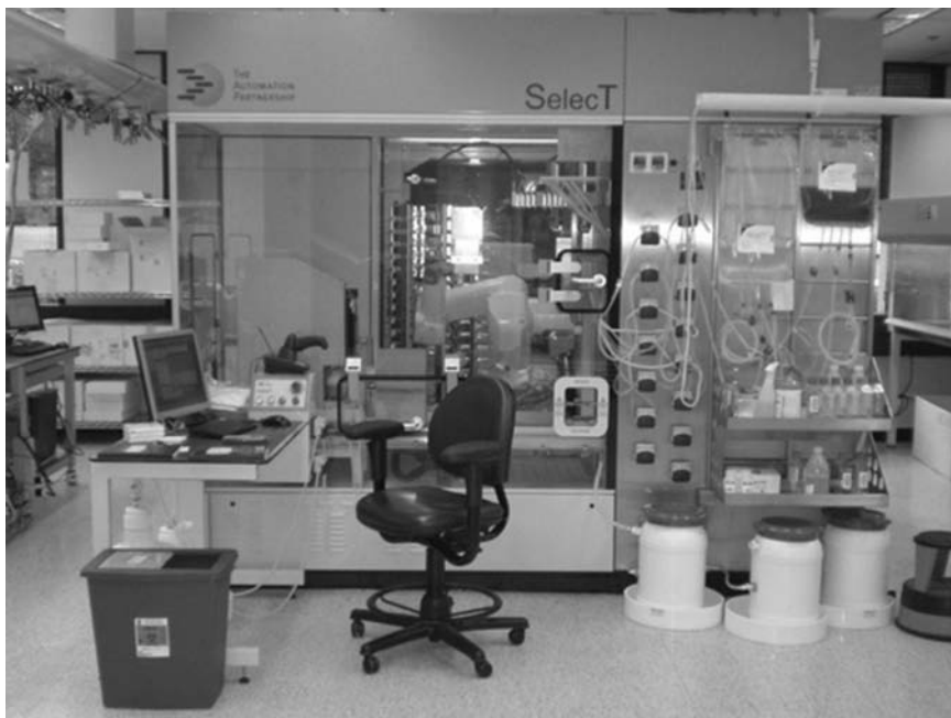
FIGURE 3 Photograph of the Select TM robot built by The Technology Partnership, Cambridge, U.K. This robot maintains between 1 and 50 cell lines, performs passaging, cell counting and viability measurements, and direct plating into microtiter plates for bioassay.
