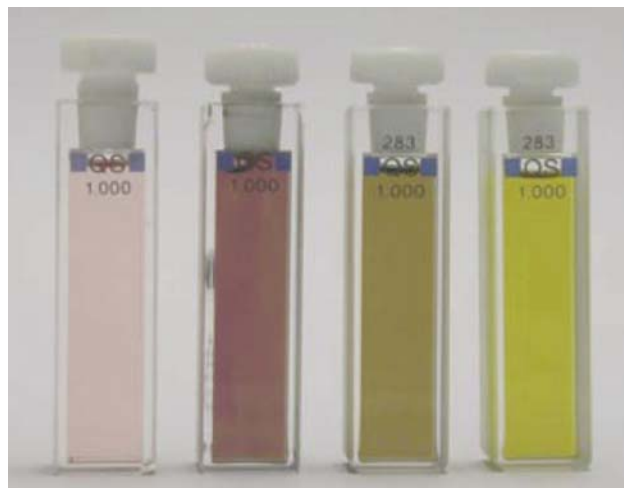
Figure 2.32 Colors shown by dichloromethane solutions of the different oxidation states of the radical 18 . From left to right: H- 18 , [K( 18crown-6 )] + 18 - , 18 and 18 + BF 4 - . (Adapted with permission from [15]. Copyright Wiley-VCH Verlag GmbH & Co. KGaA.)
