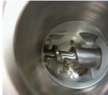
Figure 3.17 Hopper with an auger facility
