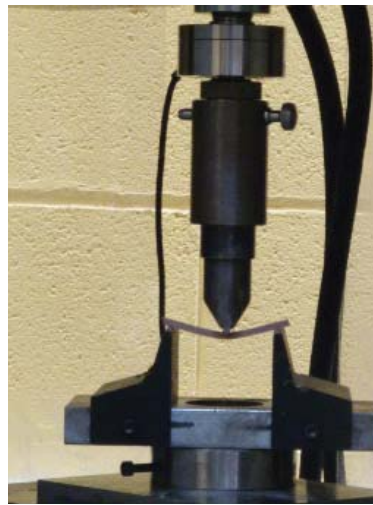
Figure 6.14 A specimen tested in 3-point bending
