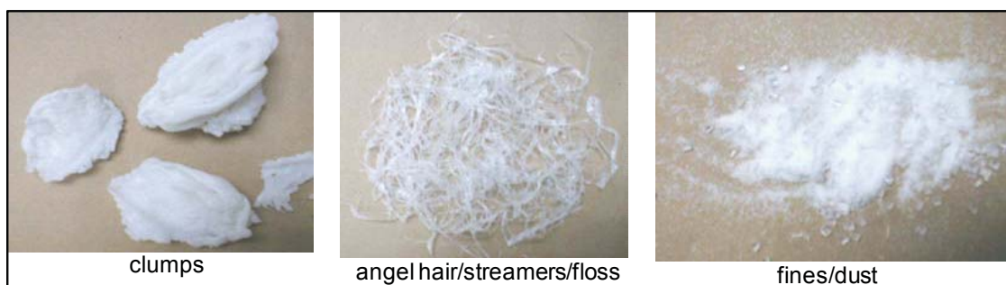
Figure 3.3 Types of degradation in delivery/conveying
