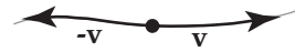
Fig. 1.5. The opposite -\mathbf{v} of an ‘autovector’ \mathbf{v} is the ‘autovector’ opposite to \mathbf{v} , and with the same absolute variation of affine parameter as \mathbf{v} (or the same length if the manifold is metric).
