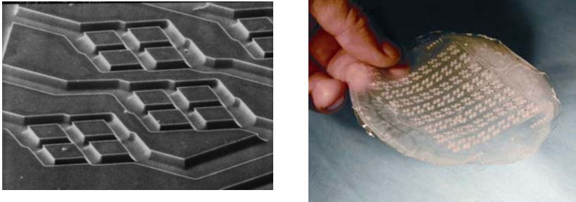
Figure 20. Silicon mold for a microfabricated capillary bed (left) and biodegradable vascular network (right) (10).
