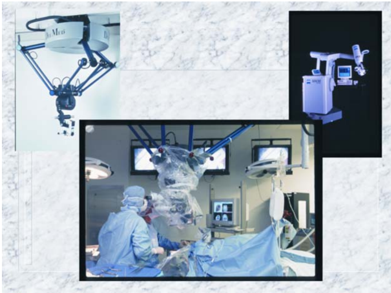
Figure 1. Upper images showing ceiling and floor stand-mounted robotic microscope used for image-guided navigation, with the lower image of a neurosurgeon and his assistant in the operating suite planning and resecting the tumor seen in Figure 2.
