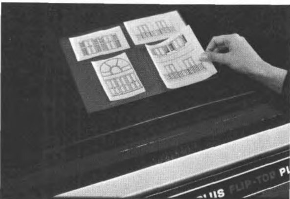
Fig. 3-27. The original tracing is reproduced in multiple. Various possible components are created and then copied onto sepia line diazo polyester.
