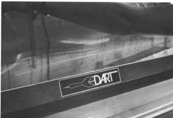
Fig. 7-3. Develop the print sheet in the ammonia developer of the diazo print machine and you'll have a screened shadow print. If you want, you can combine that screened image with an overlay sheet and make a new print showing a combination of screened base sheet and solid-line overlay.
