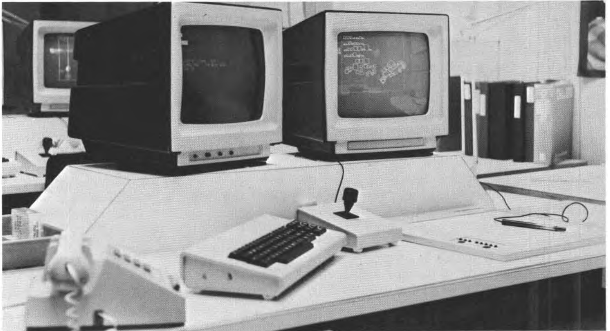
Fig. 12-1. A CADD workstation. The terminal screen on the left provides a directory of commands and prompting data; the terminal screen on the right displays the graphics.
