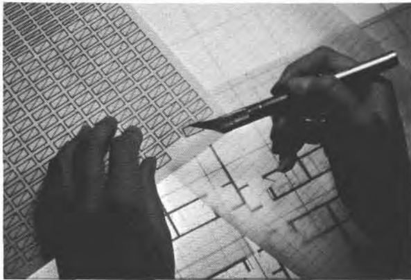
Fig. 3-23. This particular sequence is a hybrid. It's a combination of paste-up drafting on an overlay sheet. Now we're adding another systems element to the package— ap- pliqué drafting.
