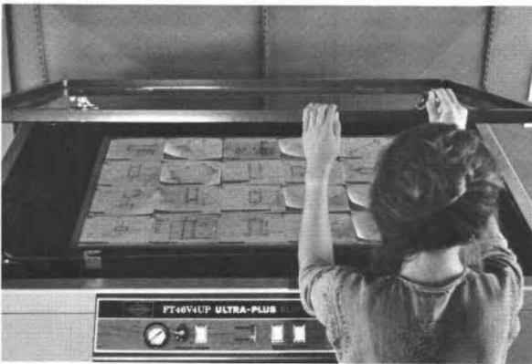
Fig. 20-14. The lid is pulled down onto the bed of the vacuum frame. The operator has to watch for displacement of original and print sheet, for bent pieces of paste-up sheet, etc. Exposure times for various print media in combination with various types of originals have been recorded and are usually on a chart next to the vacuum frame.
