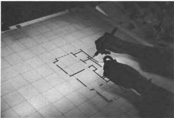
Fig. 3-2. Tape drafting is faster than hand drafting when dealing with thick lines or complex dot-dash lines. It takes some practice to bring the speed up, and drafters have to learn not to slow themselves down by cutting tiny wall pieces such as nubs for door jambs. Small items like that should be drawn with ink instead. (Most ink for technical pens will adhere to clear polyester, surprisingly enough. The inking has to be done carefully though.)
