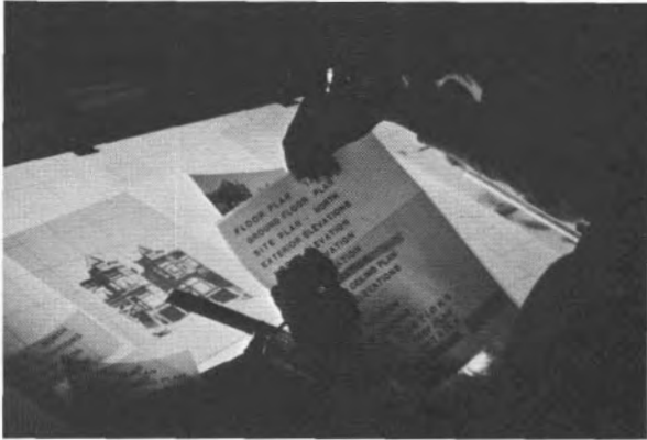
Fig. 5-6. The sepia line polyester film copy of the photocopy is resting on the light table. The graphic work assistant is selecting titles and other appliqué drafting products and tools to be used to make this photo drawing.
