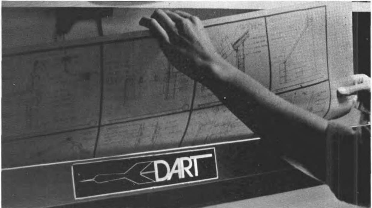
Fig. 20-16. The exposed print medium has been developed in the ammonia developer portion of a standard diazo print machine. To further intensify the image and remove traces of background emulsion, rerun the sheet through the ammonia developer and then reexpose it to ul-
