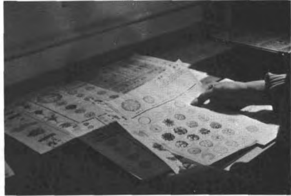
Fig. 3-45. Many designers now produce complete rendered presentation drawings by doing paste-ups of rendering components such as trees, shadows, material textures, human figures, etc., on overlay sheets atop plain line drawings of design development plans and elevations. That leaves the plans and elevations clean and clear for potential direct reuse in working drawings.
