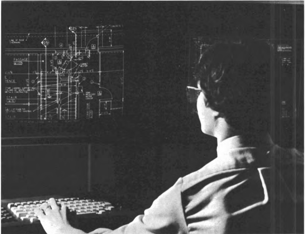
Fig. 10-2. Computer terminal with CRT for inputting and manipulating drawing data. (Courtesy of Everett I. Brown Co.)
