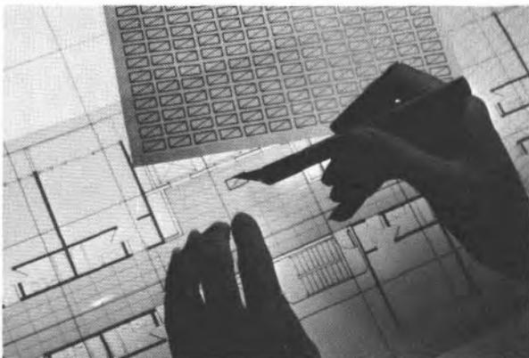
Fig. 3-24. Many architects and engineers now have small elements that are used over and over again, such as these light fixtures, printed on die-cut acetate stickyback films. Since they're pre-cut, you only have to peel them off individually and stick them in position. If there's a change later, they're easily repositioned. Most of the applique products companies can make such custom sheets for you for quantity printing.
