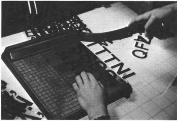
Fig. 3-40. The sepia diazo film copies of the letters are cut out for filing by the graphic work assistant.
