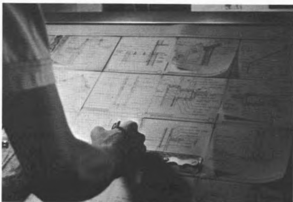
Fig. 20-12. It's generally best to hold off making a reproducible until the very end of a job and then do any final revisions on that sheet. Otherwise, keep all additions, deletions, and revisions on the original paste-up.
