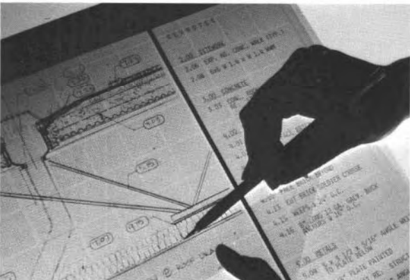
Fig. 5-14. The keynote list is spliced into the working drawing paste-up sheet. Some space is provided if it's necessary to letter-in notes by hand later. The notes are clustered and numbered according to the CSI specification divisions.
