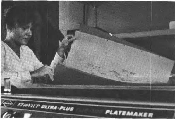
Fig. 7-4. Here's a way to get a screened background or base sheet image and solid-line overlay on the same print sheet in one general operation.
