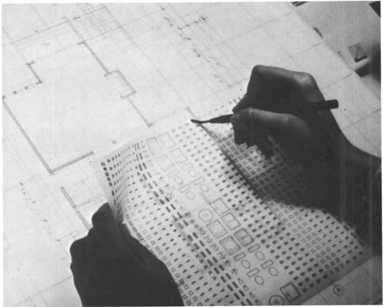
Fig. 5-1. Dry transfer, or "rub on," used for small, often used electrical and plumbing symbols.
