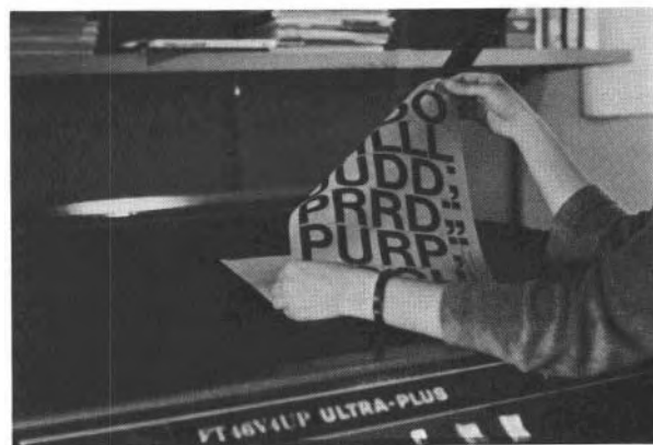
Fig. 3-39. Large rub-on, dry-transfer letters, numbers, and symbols are often hard to apply accurately or hard to apply without damage. This firm takes sheets of favored type styles and copies them on the vacuum frame onto sepia line film.
