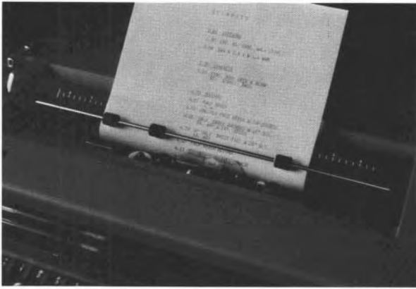
Fig. 5-12. Typewritten notation doesn't require any but normal office equipment when you use translucent paste-ups . Here, a list of keynotes is typed on regular tracing paper with an electric correctable typewriter using a film ribbon.
