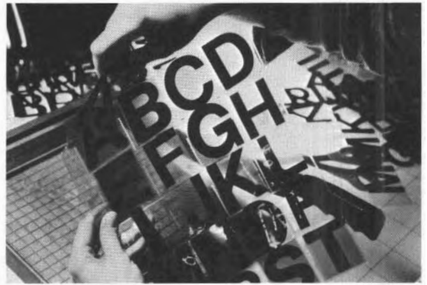
Fig. 3-41. The letters are stored in three-ring binder vinyl-pocket sheets which are distributed to all design and drafting staff.
