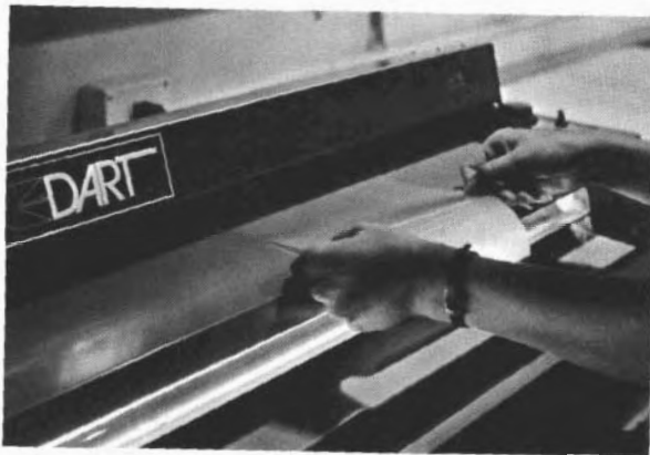
Fig. 20-4. When a detail is judged to be done enough to consider for possible reuse in a standard detail library , that's its copy stop point. At this point two draftable re-producible prints are made. The original is set aside, and drafting that's unique to the job at hand is added to one of the copies . The other copy is considered for inclusion in the detail file. Here a sheet of sepia line polyester print media has been exposed to the detail and is being fed into the ammonia developer portion of the diazo print machine.
