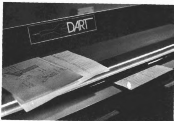
Fig. 20-5. The rotary machine has a slight effect on size fidelity in printing, but that's not considered a problem in construction details. What may be seen as more of a problem is the slow speed required to make sepia diazo polyester copies. A vacuum frame may be preferred both for size accuracy and for speed of reproduction.
