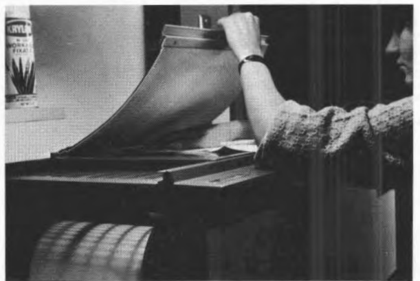
Fig. 3-43. The opaque originals are placed on the copy bed. Architects and engineers find data such as building code sections, elements from old prints, road maps (for vicinity maps), photos, rendering entourage as from Ernest Burden's book of trees, cars, people, etc., and copy them onto clear films for cutout, filing, and later paste-up.
