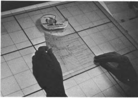
Fig. 20-10. When a detail is selected for paste-up, it's copied on the sepia line film and taped in position with transparent tape onto the polyester carrying sheet.
