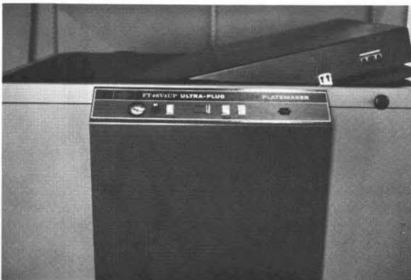
Fig. 20-15. This is a "flip-top" vacuum frame. The glass top copy bed flips over so that the print sheet and original transparency material can be exposed to a powerful ultraviolet light source inside the box.
