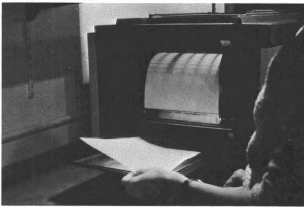
Fig. 5-3. Plain-paper copiers will copy onto tracing paper or vellum as well as onto regular bond copy paper. Here a 16-weight sheet of ordinary tracing paper is inserted in the paper feed of the copier.
