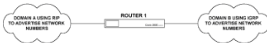
Figure 4-23: An internetwork where the use of redistribution is appropriate
