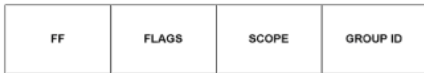
Figure 4-31: Format of an IPv6 multicast address.
