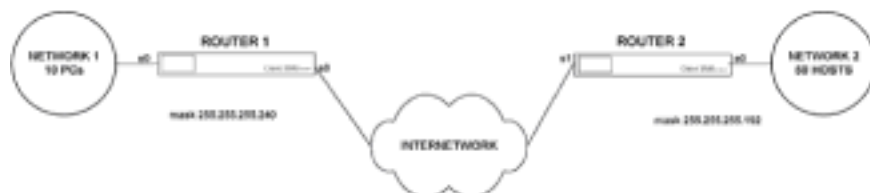
Figure 4-11: Internetwork in which VLSM is used
