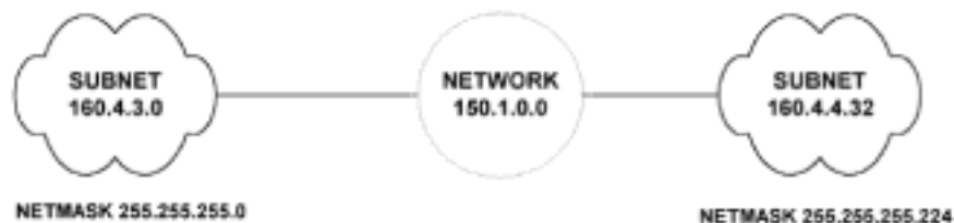
Figure 4-19: Variable-length subnet masks in OSPF
