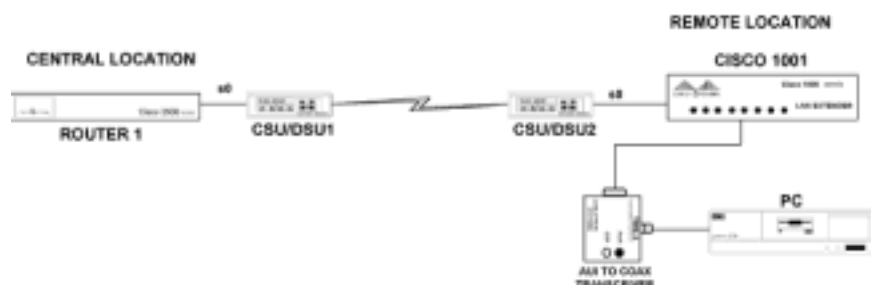
Figure 6-21: LAN extender network connections
