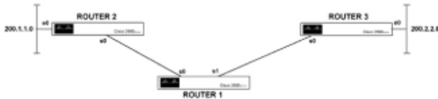
Figure 6-15: Configuration of a test X.25 network
