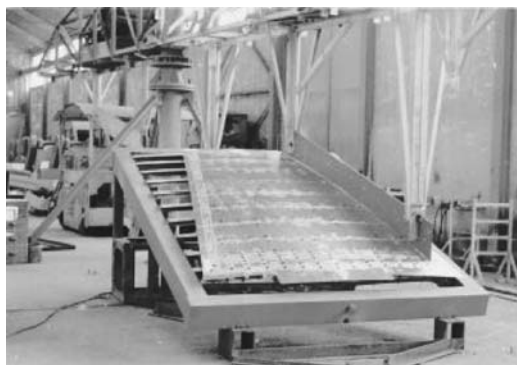
Figure 3. Panel tool being shaped by sweep boom template.
