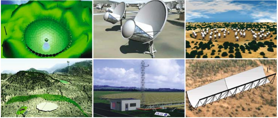
Figure 3. SKA concept visualizations. The left panel shows two large adaptive reflector ideas, one based on a 200 m diameter Arecibo-like spherical reflector (upper), the other using a much flatter reflector and an aerostat-mounted focus cabin. The middle panel (upper) shows offset paraboloids, the proposed 12 m versions being similar to the 6 m ATA antennas shown; the lower illustration shows an SKA station using aperture arrays. The right panel (upper) shows a station based on 64 \times 7 m diameter Luneburg lenses; the lower visualization is of a station employing a single 110 \text{ m} \times 15 \text{ m} cylindrical reflector. The concepts originate in China, Canada, the USA, Europe and Australia (both right hand panels). Not shown is a 12 m symmetrical paraboloid concept proposed by the Indian SKA group.
