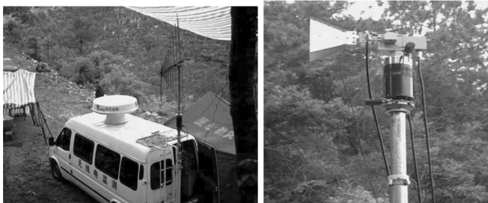
Figure 3. Photos of the log periodic antenna HL023A2 and the ETS-3115 horn antenna used by the RMSG survey group in May 2004 at Dawodang.
