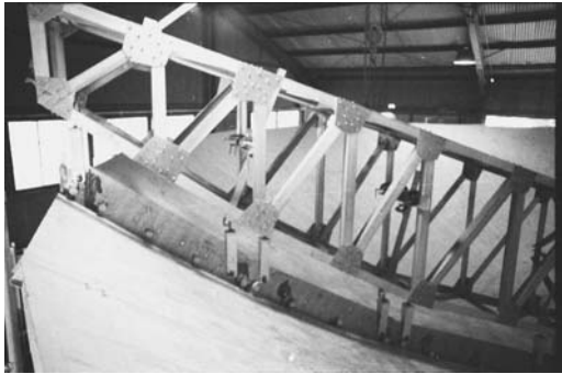
Figure 11. Sometimes reflectors were aligned by a sweep boom in the factory.
