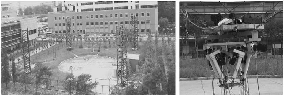
Figure 5. Field model of 50 m, including four steel towers, cable network, trolley, orientation mechanism and stabilizer.
