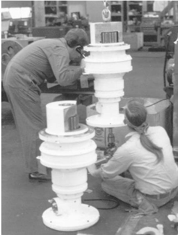
Figure 25. Planetary drives for 15.5 m antenna of Figure 1 being tested for smoothness.
