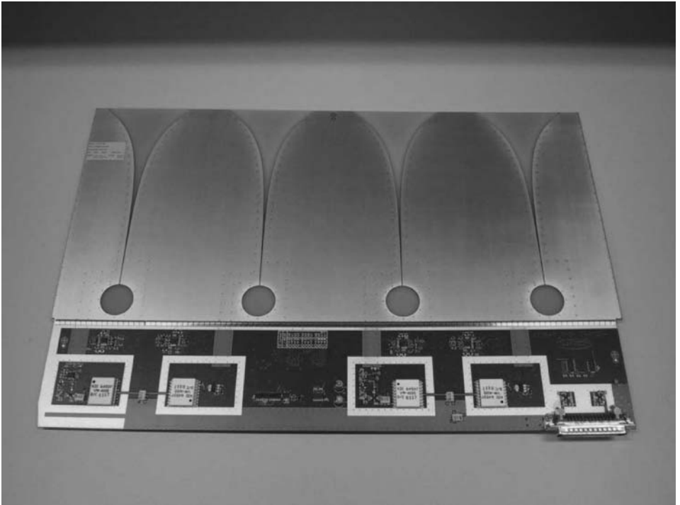
Figure 2. Picture of one of the THEA boards, showing four Vivaldi antennas and electronics.
