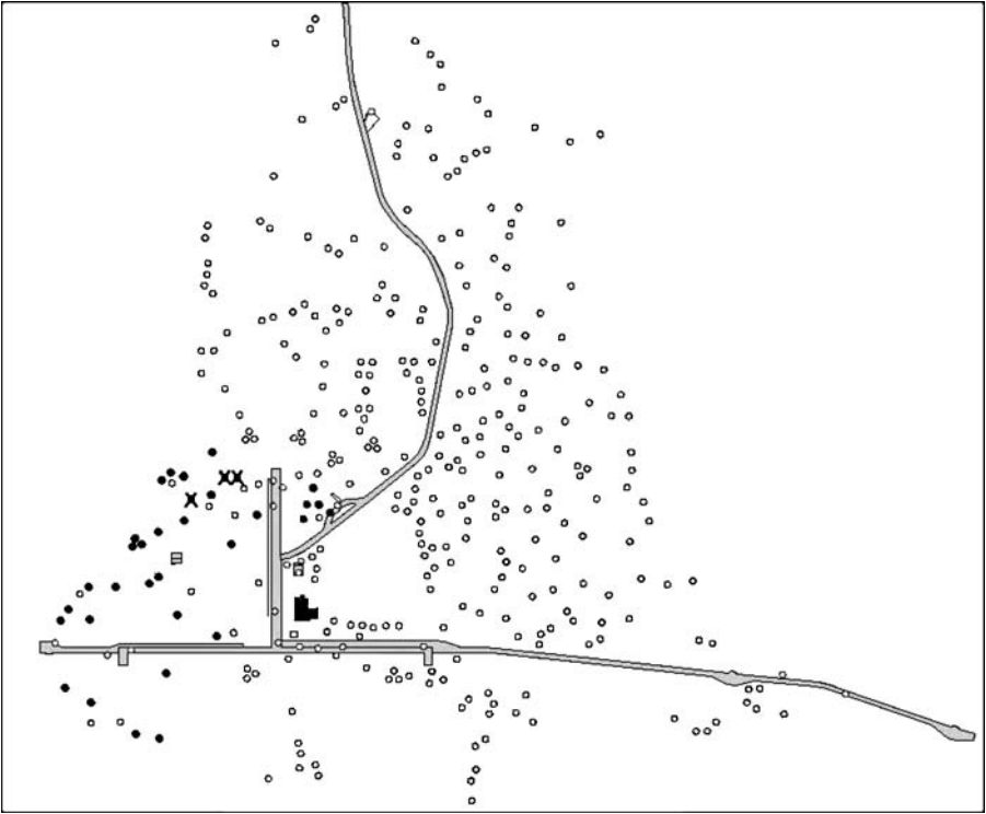
Figure 10. ATA configuration, roads and buildings at the Hat Creek Radio Observatory. The filled circles are the first 33 that are currently being emplaced and the three with the 'X's are the existing antennas. Existing accessways and buildings are also shown.
