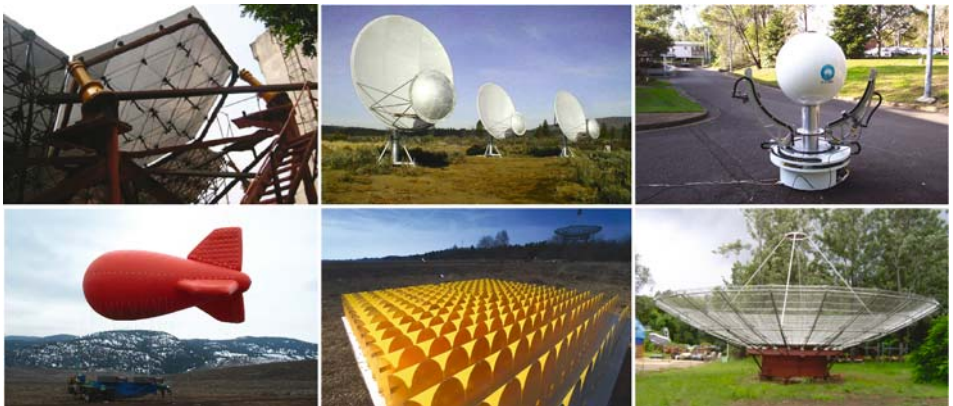
Figure 4. SKA technology prototypes. At left are components for large reflectors. The upper panel shows a prototype deformable surface for the FAST demonstrator while the lower panel illustrates a test aerostat for the suspended-feed LAR concept. The middle panel shows three 6 m dishes of the ATA (upper), together with a patch of an aperture array demonstrator based on Vivaldi-notch end-fire elements (lower). At upper right is a 0.9 m Luneburg lens with a two-arm feed translator. The lower right panel shows a prototype 12 m dish constructed using a mesh surface and pre-loaded radial members.
