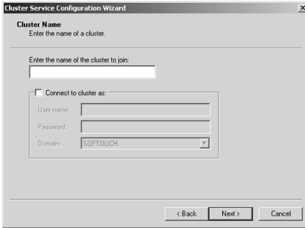
Figure 18.2 Additional nodes in a cluster are added by installing the cluster service on the additional machines and specifying the name of the cluster that is being joined.
