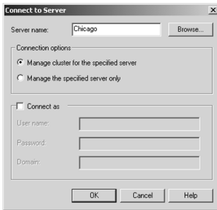
Figure 9.3 In creating or joining a cluster, you provide the security credentials to use when connecting to the server that is running Application Center 2000.
