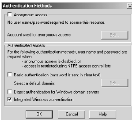
Figure 16.2 From IIS it is possible to configure Integrated Windows authentication to authenticate Web users on the basis of the .NET Active Directory structure.
