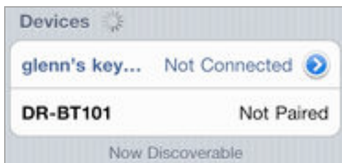
Figure 24: The keyboard is paired but not connected; the DR-BT101 (a set of headphones) is not yet paired.
