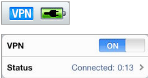
Figure 92: The status bar shows an active VPN connection (top), while the VPN view shows how long you've been connected (bottom).
