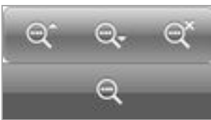
Figure 71: The magnifying glasses with up arrow (for back) and down arrow (for forward) step you through matches. Tap the glass with an X in the corner to cancel the search.
