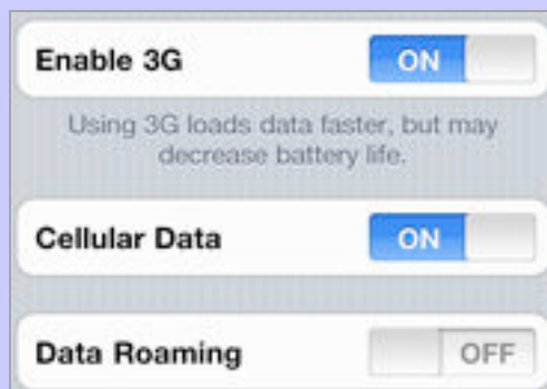
Figure 3: The Enable 3G switch lets you toggle high-speed—and high-battery-use—mode on and off, whereas the Cellular Data switch lets you turn all mobile broadband access on or off separately from Wi-Fi networking. Data Roaming affects use outside your home country.
