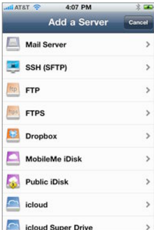
Figure 49: Air Sharing Pro offers a cornucopia of server types, including three flavors of FTP, MobileMe, Dropbox, a few hosting services, generic WebDAV, and Mail Server access (POP and IMAP).
