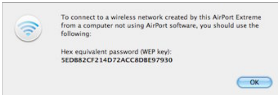
Figure 4: The Network Equivalent Password dialog gives you the hex key value of a text network key.
