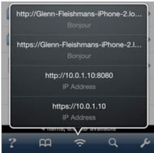
Figure 59: The various ways to connect over a local network appear when you tap the Wi-Fi icon.
