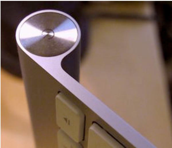
Figure 28: The power button is located on the right upper side of the Apple Wireless Keyboard.
