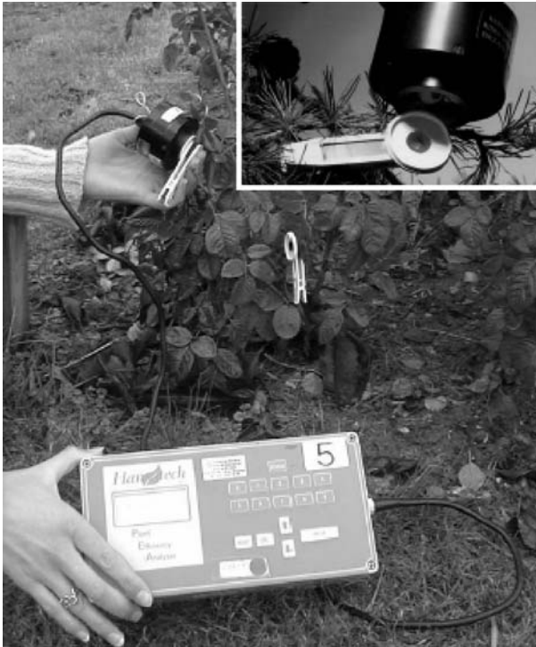
Fig. 21.3 The PEA (Handy-PEA) fluorimeter used for our studies. The photo is from in situ measurements, with the clips already put on the leaves to dark-adapt them. The insert shows the sensor of the instrument, which provides, by LEDs, the red actinic light (650 nm) and collects the fluorescence signals
