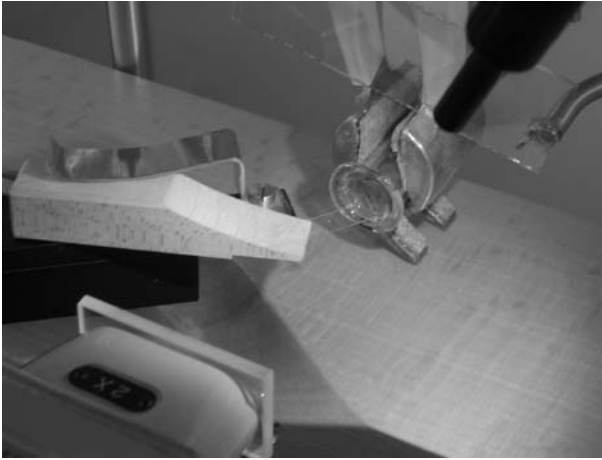
Fig. 17.1 Transfer platform for small samples fixed in front of the quartz fiber balance housing
