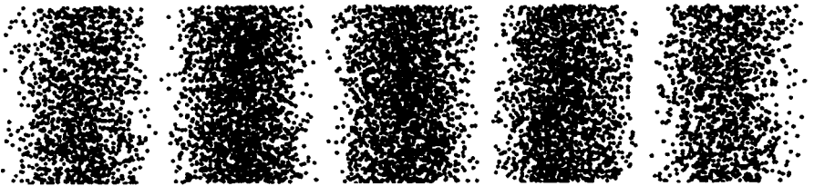
Fig. 1.3 A computer generated simulation of the build-up of a two-slit interference pattern. Each dot records the detection of a quantum particle on a screen positioned behind two slits. Patterns formed by 100, 1000 and 10000 quantum particles are illustrated.
