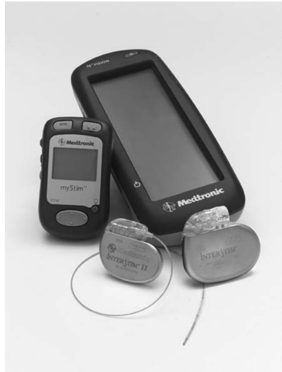
Figure 26.7 Patient programmer with control magnet. Physician programmer also viewed. (Reprinted with the permission of Medtronic, Inc. © 2006). (See also color plate section).
