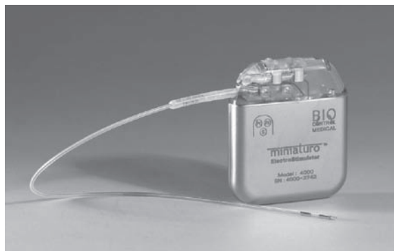
Figure 28.1 The Miniatur TM -I electrostimulator (4 × 5 × 0.8 cm) with electrode connected.
