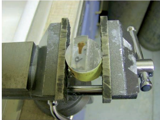
Fig. 4 An embedded bone block that has been trimmed for sectioning
