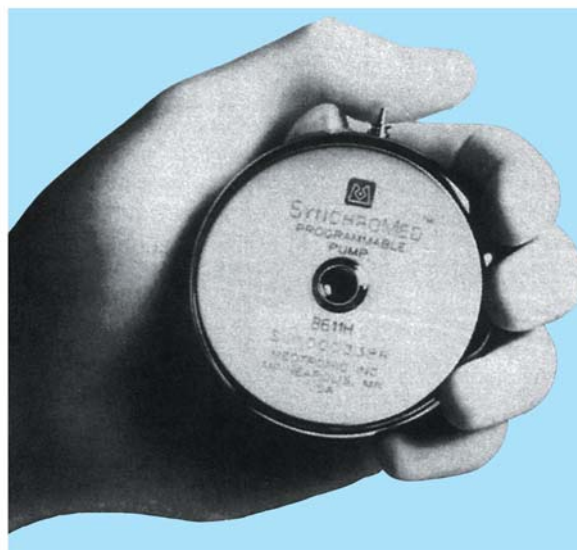
FIGURE 17-5 ▼ An example of an implantable, electronically controlled PCA pump. This pump is implanted surgically in the patient's abdomen and can be refilled periodically through a self-sealing septum.
