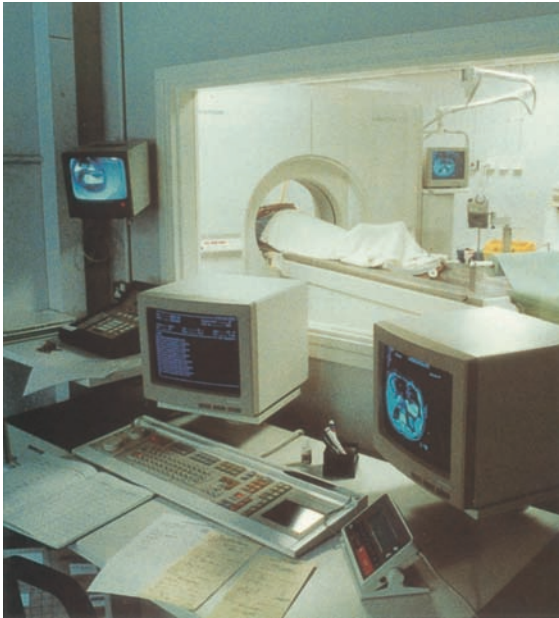
Figure 5.17 Computed tomography (CT) scanner (Siemens Somatom Plus). Courtesy of Ms Linda Banks
