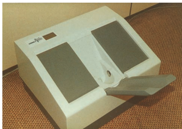
Figure 5.25 Apparatus (Lunar Achilles) for ultrasound measurement of the calcaneus. Courtesy of GE Lunar, Madison, WI
